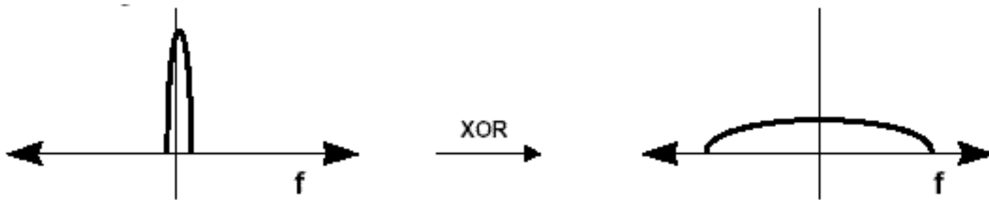
Figure 5a Effect of PN Sequence on Transmit Spectrum
