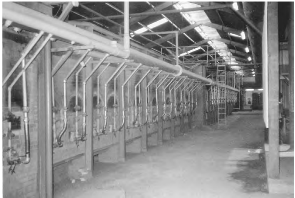
Figure 2-5 Tunnel kilns provide even heat distribution.
