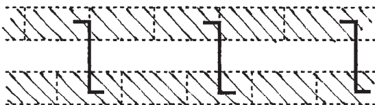
rigid "Z" ties (for use with solid units only)
