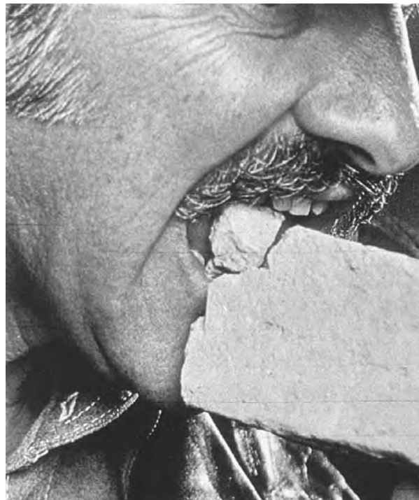
Figure 3-4 Substandard brick. (Photos courtesy Brick Institute of Texas.)
