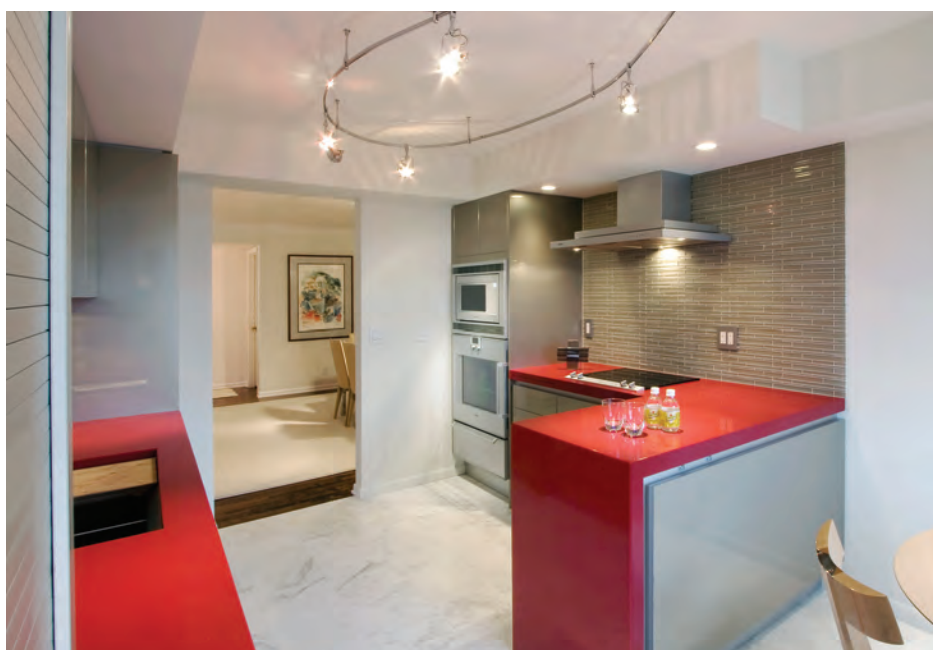
FIGURE 7.16 General or ambient lighting is provided by low-voltage lighting on a cable at the ceiling.
