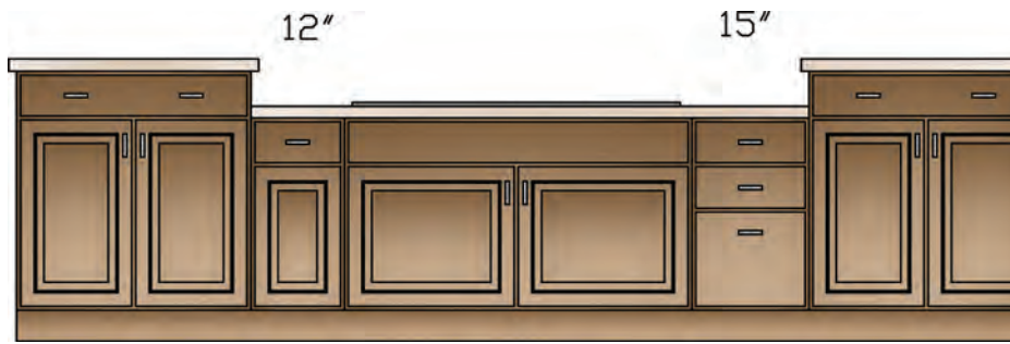
FIGURE 8.31 Guideline 17: A cooktop and the adjacent landing counters must be at the same height.
