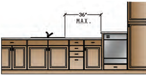
FIGURE 6.28 Locate nearest edge of the primary dishwasher within 36 inches (914 mm) of the nearest edge of a cleanup/prep sink (Kitchen Planning Guideline 13).
