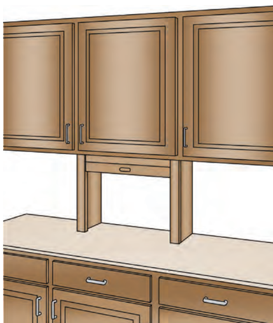
FIGURE 6.56 An appliance garage can be placed on the counter within the 158 inches (4013 mm) of counter space, as long as it does not interfere with landings and preparation areas (Kitchen Planning Guideline 25).
