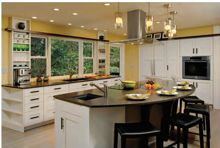
FIGURE 6.32 A second or auxiliary sink is handy for a variety of purposes. It should have at least an 18-inch (457 mm) landing area to one side and 3 inches (76 mm) of clear space on the other (Kitchen Planning Guideline 15).
