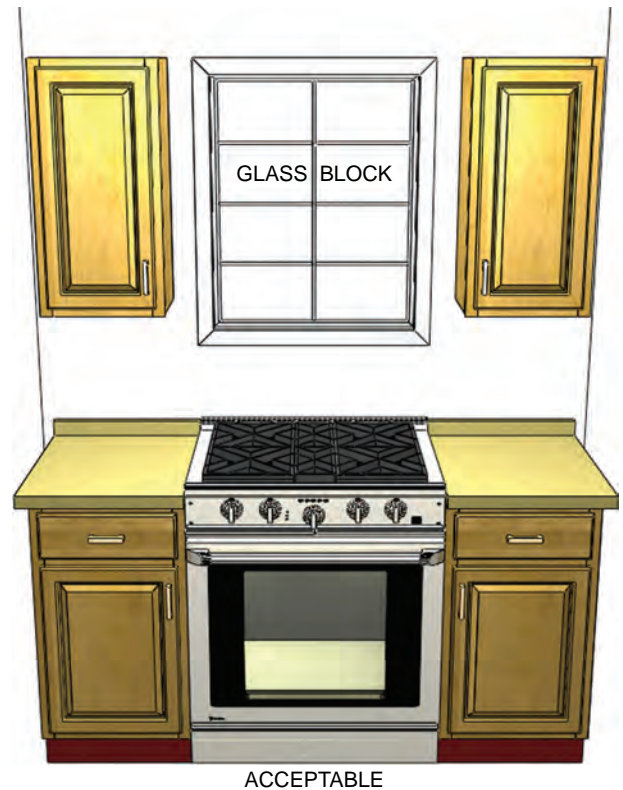
FIGURE 6.37 Placing a window behind a cooking surface may mean it is difficult to clean, but it is acceptable to put a nonoperable window behind the cooking surface. An operable window and/or a flammable window treatment would be dangerous (Kitchen Planning Guideline 20).
