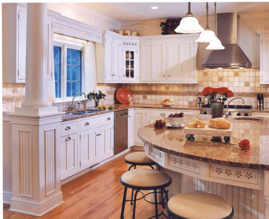
FIGURE 6.27 The cleanup sink and the dishwasher should be within 36 inches (914 mm) of each other.
