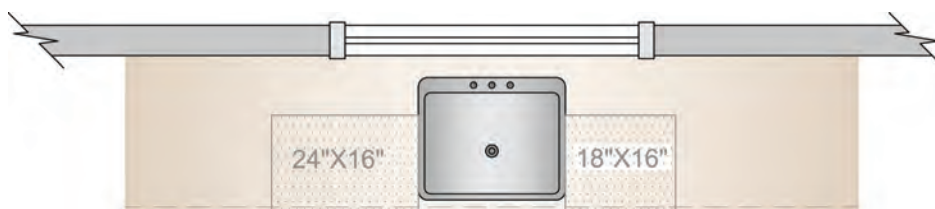
FIGURE 6.21 Plan 24 inches (610 mm) of landing area to one side of the primary sink and 18 inches (457 mm) on the other side (Kitchen Planning Guideline 11).
