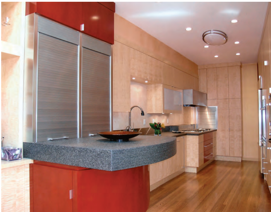
FIGURE 8.3 There is a trend toward sliding and tambour doors. These door types reduce risk of injury by staying out of the way.
