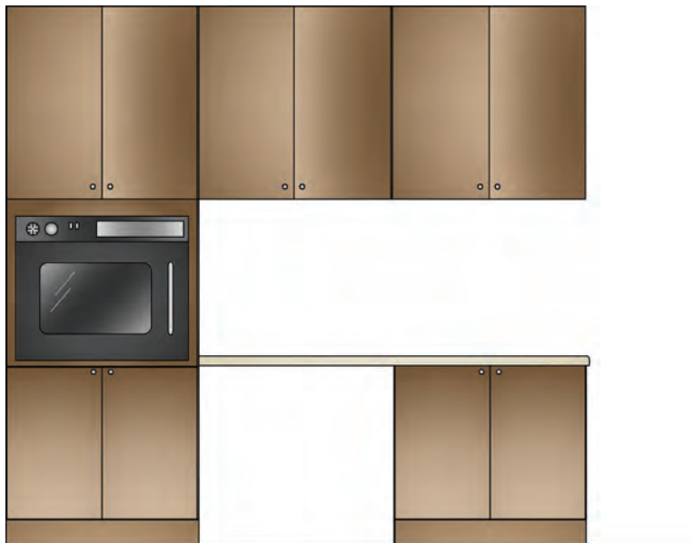
FIGURE 8.35 Access standard 23: Landing space at the oven.
