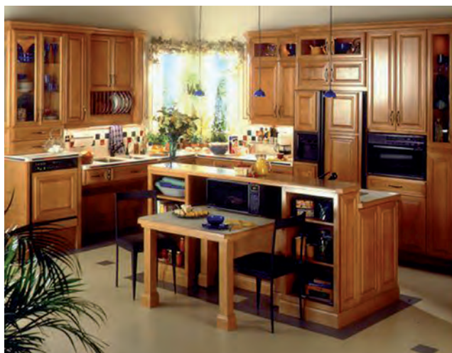
FIGURE 8.24 This raised dishwasher is placed at the end of the cabinet and counter length, making it aesthetically and functionally right. Courtesy of Mary Jo Peterson, Inc.
