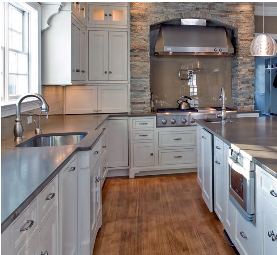
FIGURE 4.18 A microwave installed below the countertop with generous work aisles in front provides for easy approach, reach, and use.
