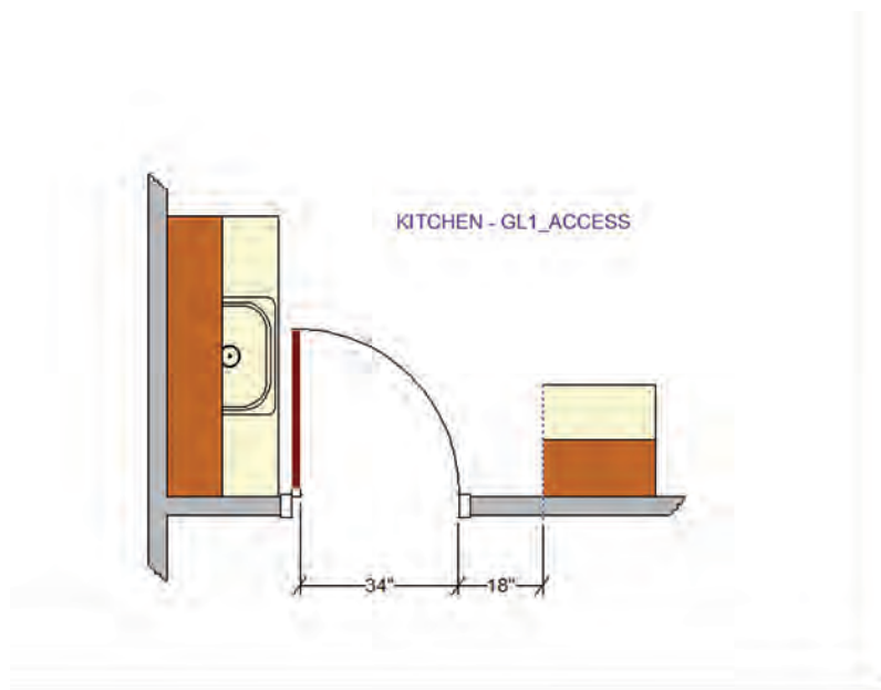
FIGURE 8.4 Access Standard 1: The clear opening of a doorway should be at least 34 inches (864 mm), requiring a 36-inch (914-mm) door to allow for passage by a person using a mobility aid, and there should be 18 inches (457 mm) of clear floor space adjacent to the latch side of the swing side of the door.
