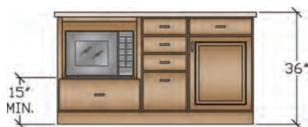
FIGURE 6.45 A microwave can be placed below a 36 inch (914 mm) high counter, when the bottom of the shelf is at least 15 inches (381 mm) off the floor (Kitchen Planning Guideline 21). This may be suitable placement for a seated user or for children.
