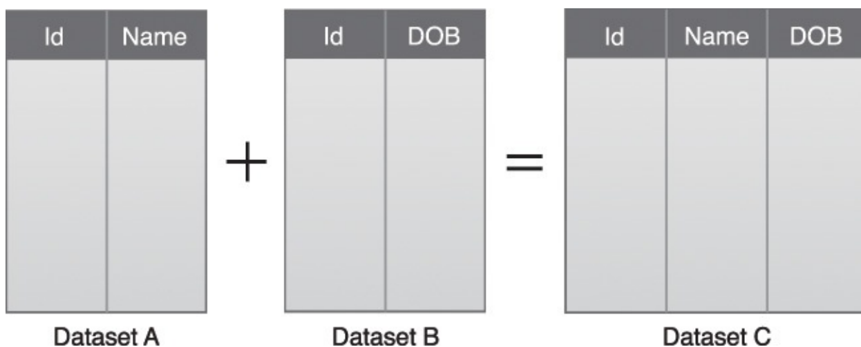
Figure 3.18 A simple example of data aggregation where two datasets are aggregated together using the Id field.
