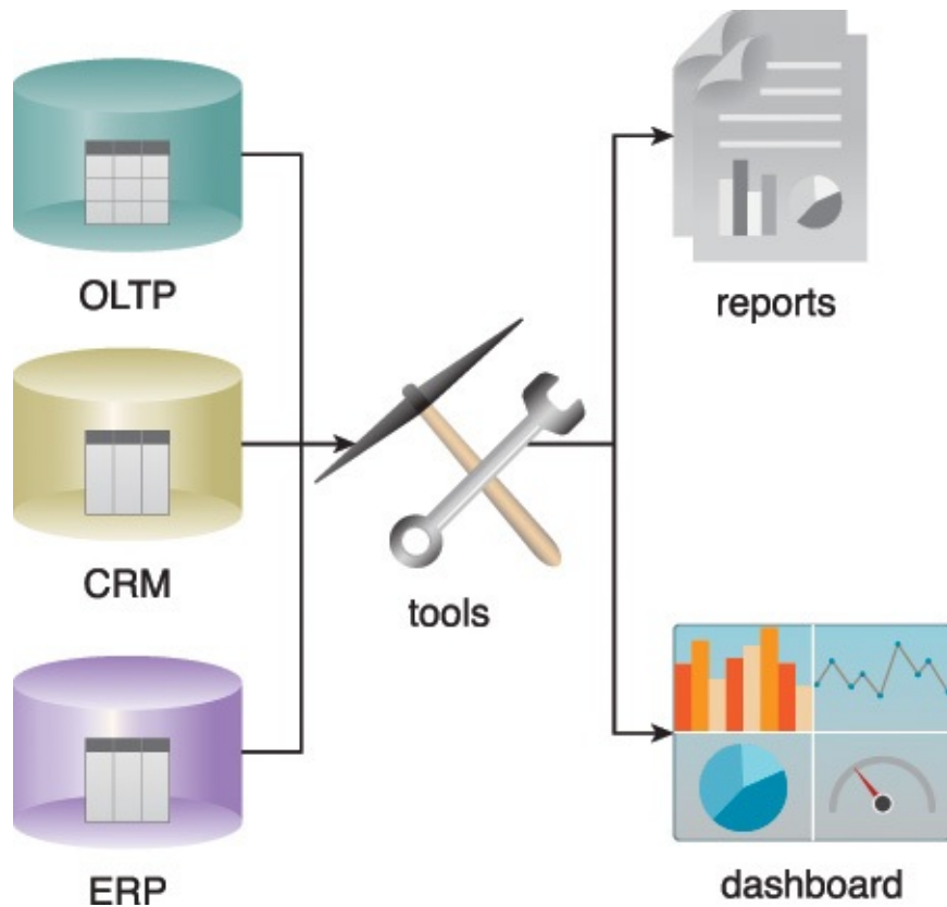
Figure 1.5 The operational systems, pictured left, are queried via descriptive analytics tools to generate reports or dashboards, pictured right.
