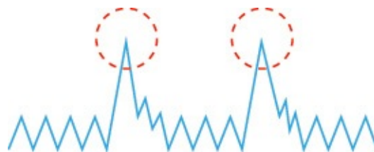
Figure 3.16 The presence of invalid data is resulting in spikes. Although the data appears abnormal, it may be indicative of a new pattern.
