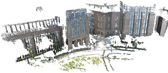
**Figure 5: 3D reconstruction using Bundler SfM.** 33K points from 47 photos of a university plaza, model post-processed for enhanced density/visual clarity.
