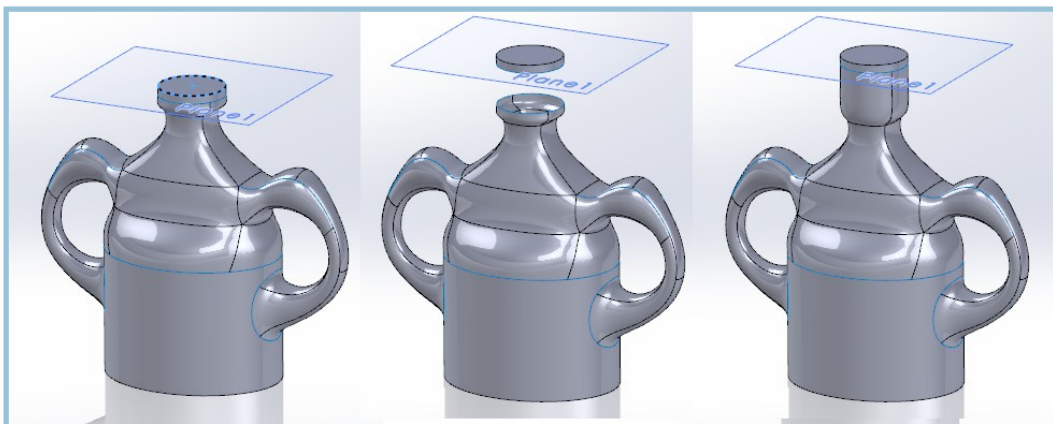
Figure 23 – The original cap position, left, moving the cap plane position up, center, only the con-
