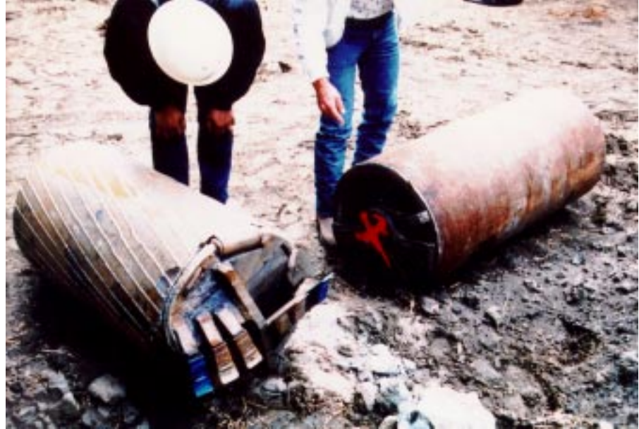
Figure 6-5: Drilling Bucket/Cleanout Bucket Comparison
