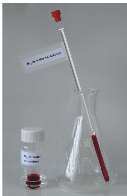
Fig. 1 Setup for vapour diffusion (left) and layering (right) exemplified with aqueous vitamin B 12 solutions (acetone as an antisolvent). In the case of the vapour diffusion, the antisolvent acetone must be refilled several times for crystal growth. The image has been edited in order to make the transparent layer of the antisolvent within the NMR tube more visible.
