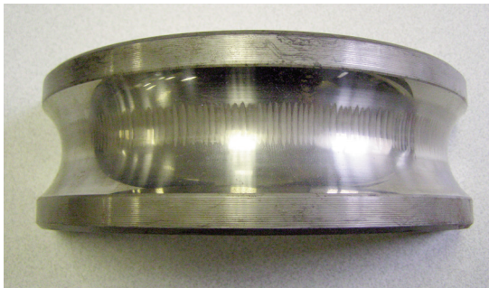
Figure 3. Damaged Bearing from ASD Induced Shaft Currents.
