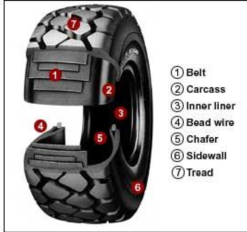
Structural Diagram of Off-the-Road Radial Tires
