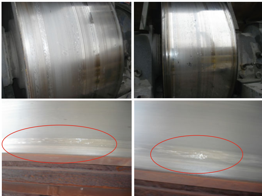
Fig. 7.37 Damages on the carrying surface of the supporting rollers and tyre due to kiln crank
