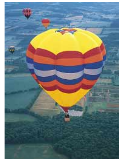
Hot-air balloons. Because hot air is less dense than cold air, a net upward force acts on the balloons.
