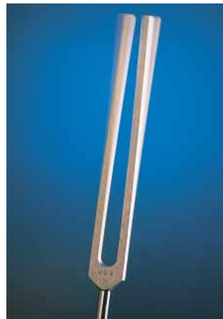
The sound from a tuning fork is produced by the vibrations of each of its prongs.
