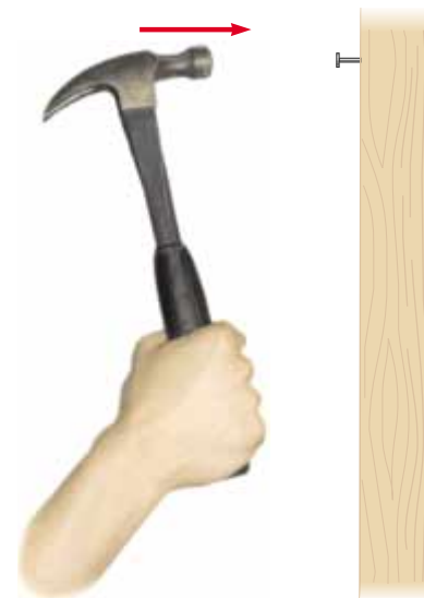
Figure 7.14 The moving hammer has kinetic energy and thus can do work on the nail, driving it into the wall.
