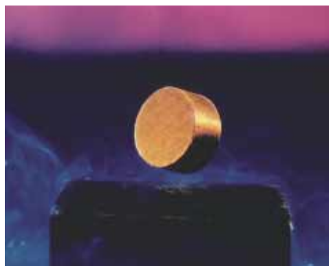
Figure 30.34 A small permanent magnet levitated above a disk of the superconductor \text{YBa}_2\text{Cu}_3\text{O}_7 cooled to liquid nitrogen temperature (77 K).
