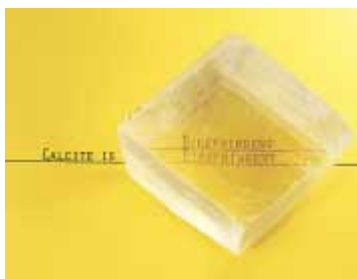
Figure 38.33 A calcite crystal produces a double image because it is a birefringent (double-refracting) material.
