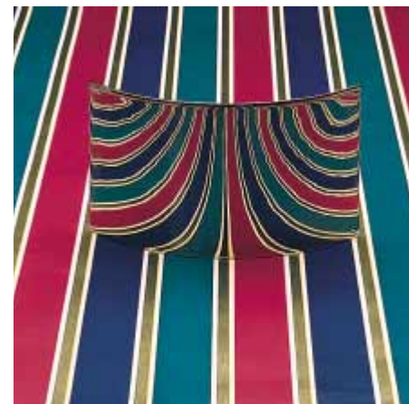
Reflection of parallel lines from a convex cylindrical mirror. The image is virtual, upright, and reduced in size.
