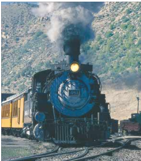
Figure 22.1 This steam-driven locomotive runs from Durango to Silverton, Colorado. It obtains its energy by burning wood or coal. The generated energy vaporizes water into steam, which powers the locomotive. (This locomotive must take on water from tanks located along the route to replace steam lost through the funnel.) Modern locomotives use diesel fuel instead of wood or coal. Whether old-fashioned or modern, such locomotives are heat engines, which extract energy from a burning fuel and convert a fraction of it to mechanical energy.
