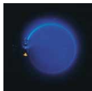
Figure 29.19 The bending of an electron beam in a magnetic field.
