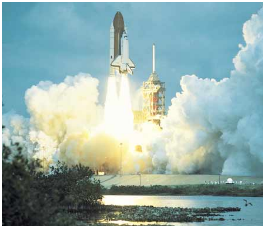
Figure 9.28 Liftoff of the space shuttle Columbia . Enormous thrust is generated by the shuttle’s liquid-fuel engines, aided by the two solid-fuel boosters. Many physical principles from mechanics, thermodynamics, and electricity and magnetism are involved in such a launch.
