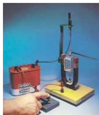
Figure 28.23 (a) The principal components of a D'Arsonval galvanometer. When the coil situated in a magnetic field carries a current, the magnetic torque causes the coil to twist. The angle through which the coil rotates is proportional to the current in the coil because of the counteracting torque of the spring. (b) A large-scale model of a galvanometer movement. Why does the coil rotate about the vertical axis after the switch is closed?
