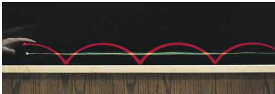
Figure 11.1 One light source at the center of a rolling cylinder and another at one point on the rim illustrate the different paths these two points take. The center moves in a straight line (green line), whereas the point on the rim moves in the path called a cycloid (red curve). (Henry Leap and Jim Lehman)
