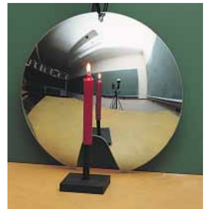
Figure 36.15 Ray diagrams for spherical mirrors, along with corresponding photographs of the images of candles. (a) When the object is located so that the center of curvature lies between the object and a concave mirror surface, the image is real, inverted, and reduced in size. (b) When the object is located between the focal point and a concave mirror surface, the image is virtual, upright, and enlarged. (c) When the object is in front of a convex mirror, the image is virtual, upright, and reduced in size.
