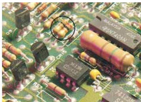
Figure 27.6 The colored bands on a resistor represent a code for determining resistance. The first two colors give the first two digits in the resistance value. The third color represents the power of ten for the multiplier of the resistance value. The last color is the tolerance of the resistance value. As an example, the four colors on the circled resistors are red (= 2), black (= 0), orange (= 10^3 ), and gold (= 5%), and so the resistance value is 20 \times 10^3 \Omega = 20 \text{ k}\Omega with a tolerance value of 5% = 1 k \Omega . (The values for the colors are from Table 27.2.)
