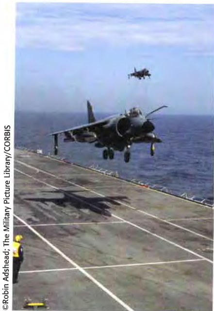
The jet exhaust of this VTOL aircraft can be vectored downward for vertical takeoffs and landings.
