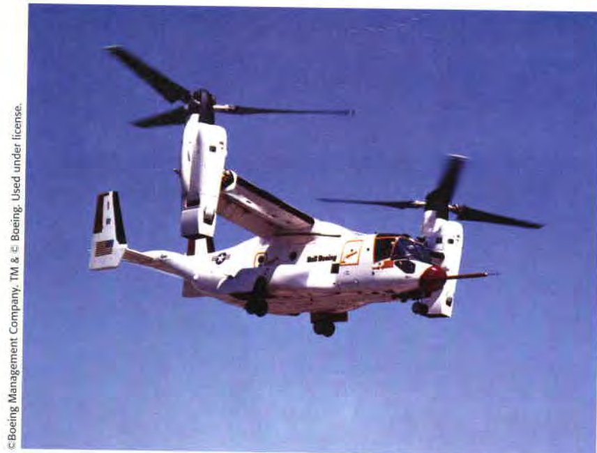
The engine/propeller units at the wingtips of this aircraft can tilt from the vertical takeoff position shown to a horizontal position for forward flight.
