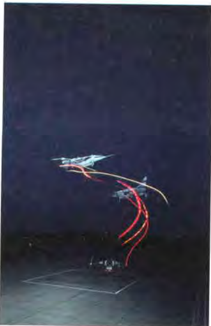
This time-lapse photo of a VTOL aircraft shows a three-dimensional combination of translation and rotation.
