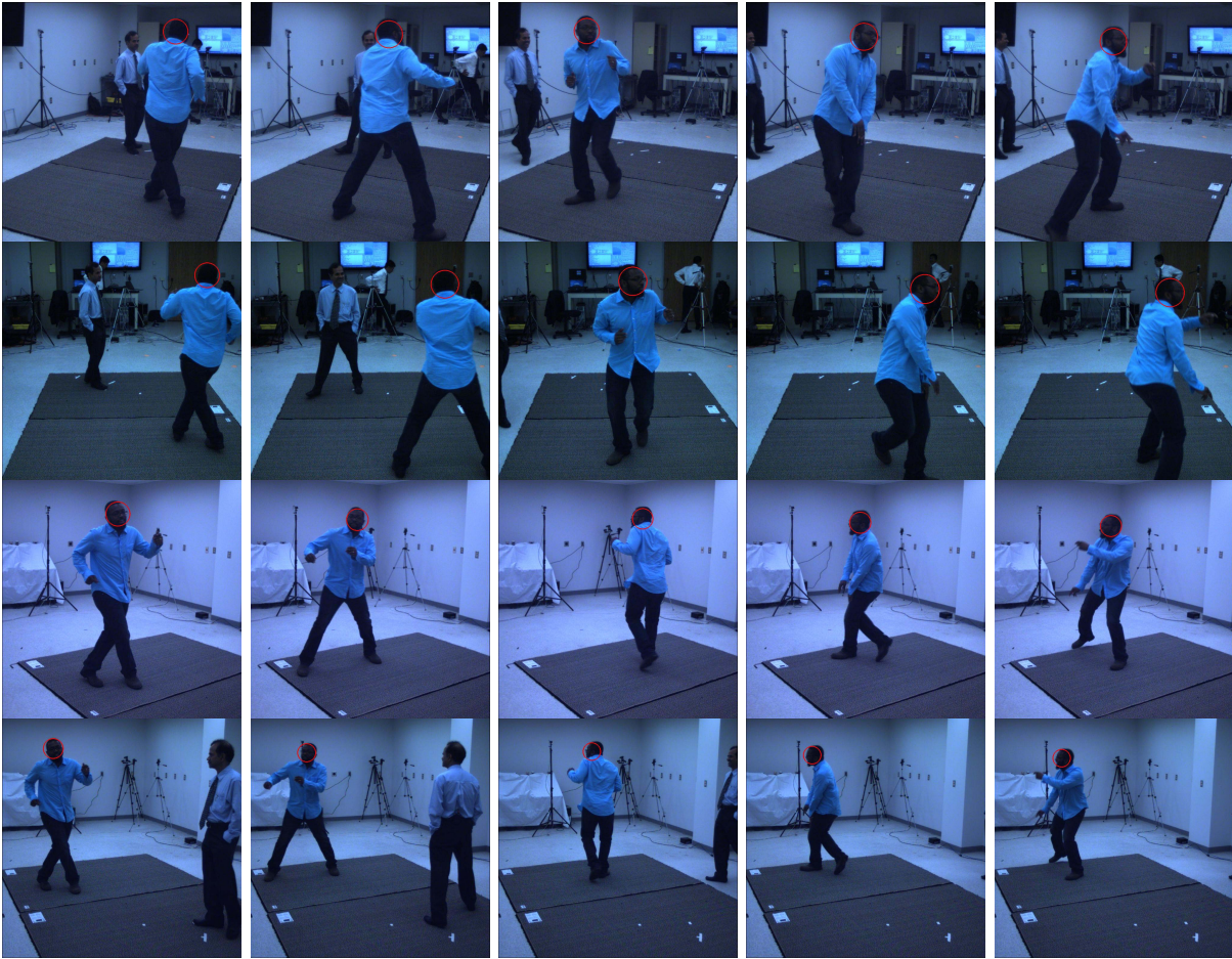
Fig. 6. Sample Tracking Results Tracking results for a 200-frame multi-view video sequence. The subject performs dramatic dancing motions. Five views are shown here. Each row of images is captured by the same camera. Each column of images is captured at the same time.
