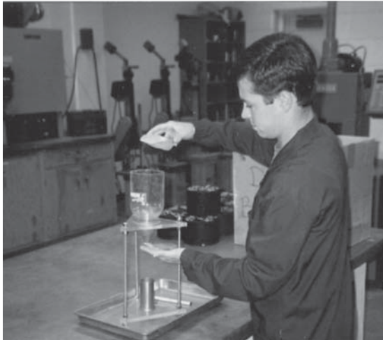
FIGURE 8.8 Testing for uncompacted voids for fine aggregates.
