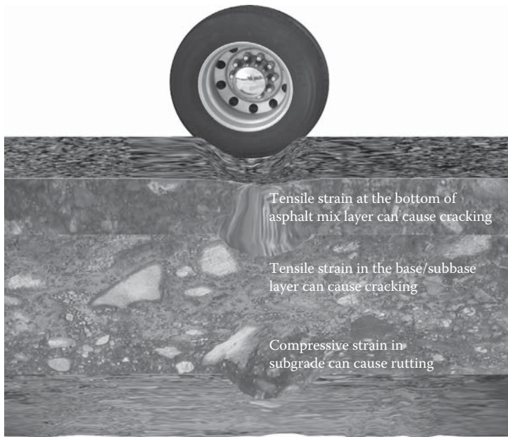
A flexible pavement “flexes” under a load; repeated loadings cause repeated compressive strains as well as tensile strains
