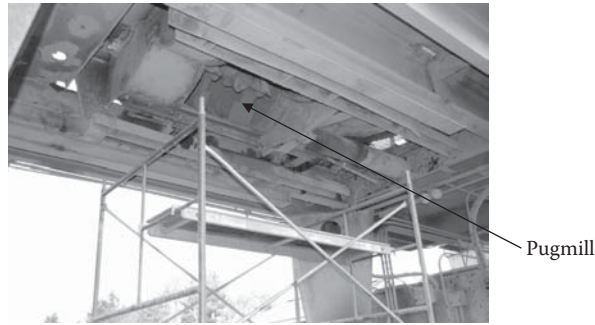
FIGURE 16.6 Pugmill, view from the bottom with discharge door removed. (Courtesy of Matthew Teto, All States Asphalt, Sunderland, MA.)
