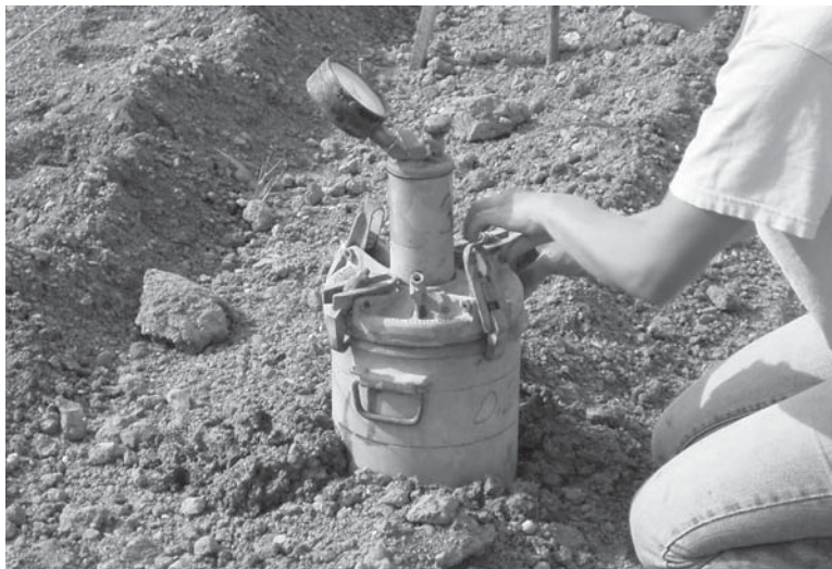
FIGURE 17.25 Field testing of air content in concrete using the air pressure meter. (Courtesy of James Cable.)
