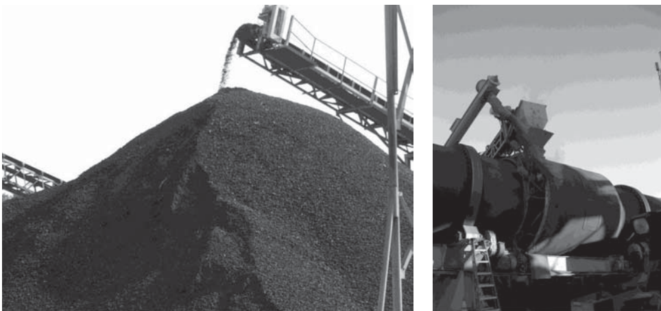
FIGURE 16.8 RAP stockpile and RAP feeding system in a drum plant. (Courtesy of Robert Frank.)
