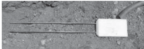
FIGURE 22.2 Time domain reflectometry (TDR) probe. (Courtesy of Lauren Swett.)
