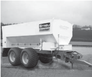
Wirtgen SW 16TA lime spreader Tank capacity: 16.5 m 3 , Spreading width: 2500 mm Spreading quantity: 2–50 L/m 2 , Manual operation spreading auger
