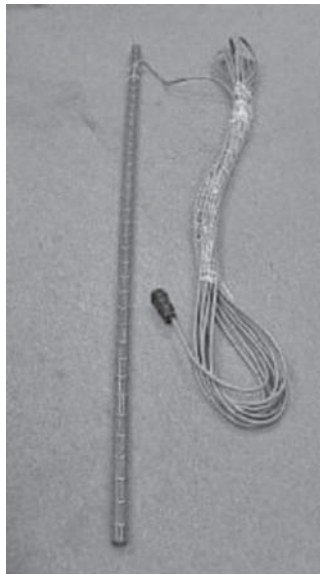
FIGURE 22.3 Frost depth measurement instrument. (Courtesy of Lauren Swett.)
