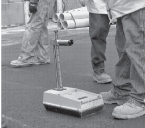
FIGURE 20.1 Schematic of backscatter operation and nuclear gage equipment gage used on HMA.
