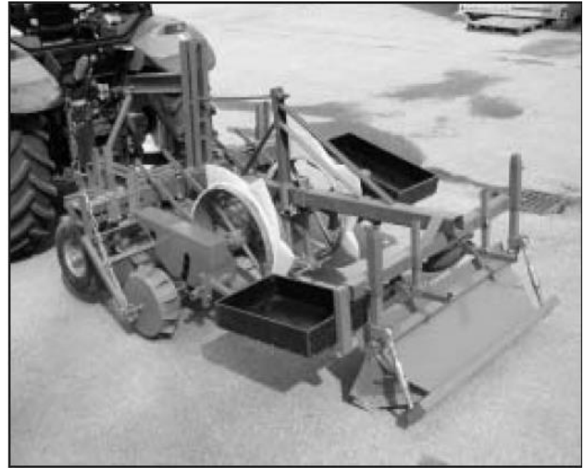
Fig. 2: Vegetable planter modified for horse radish – development stages
