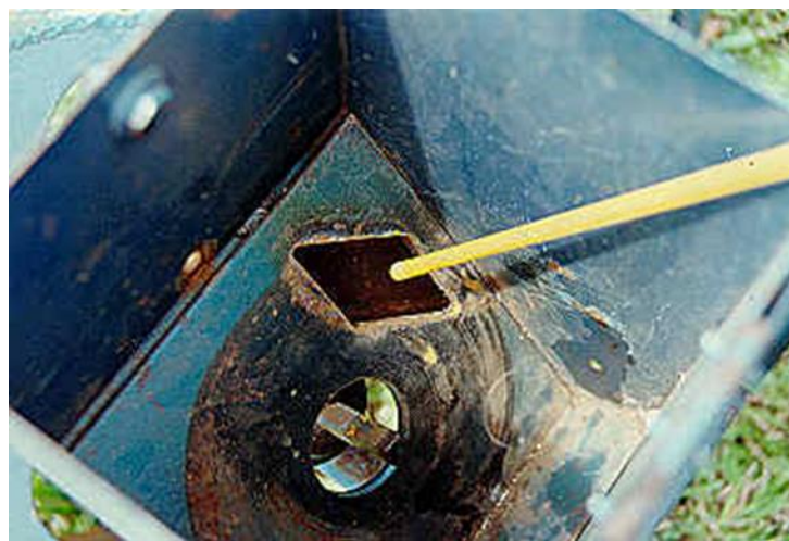
Mechanism for Pushing Seeds Out of Seed Cells
