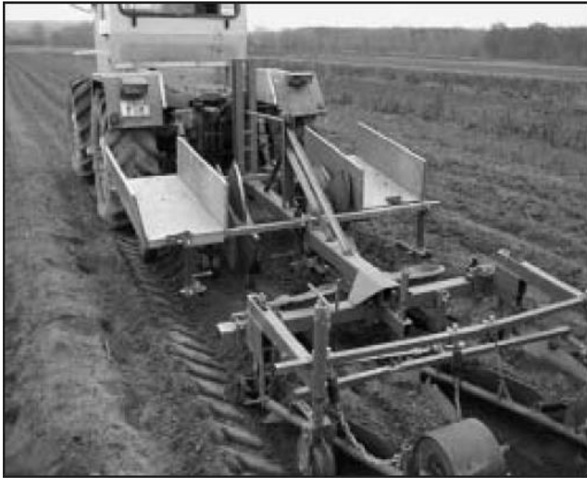
Fig. 2: Vegetable planter modified for horse radish – development stages
