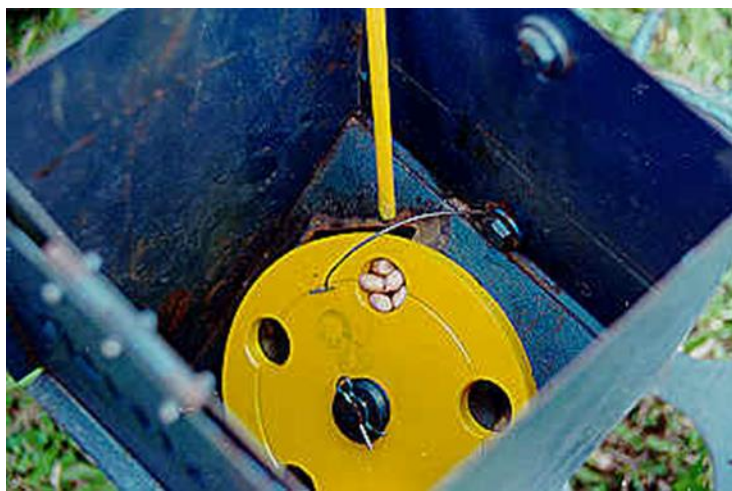
Mechanism for Pushing Seeds Out of Seed Cells
