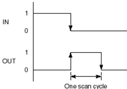
**Figure: Behavior of One-Shot (Fall Trigger)**
