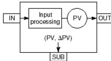
Figure: Function Block Diagram of Input Indicator Block (PVI)
