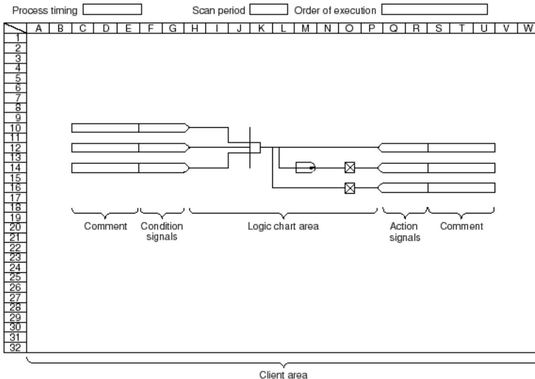
**Figure: Configuration of the Entire Logic Chart**
