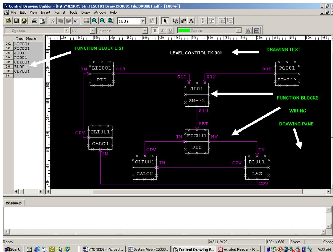
Figure: Control drawing environment
