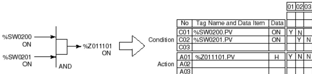
**Figure : AND Circuit Example**
