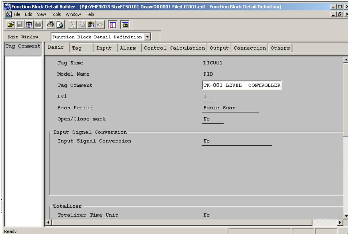
**Figure: Function block detail builder for PID block.**
