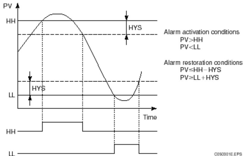
**Figure: Input High-High and Low-Low Limit Alarm Check**
