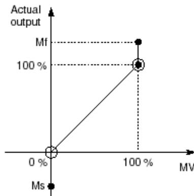
**Figure: Tight-shut function**
