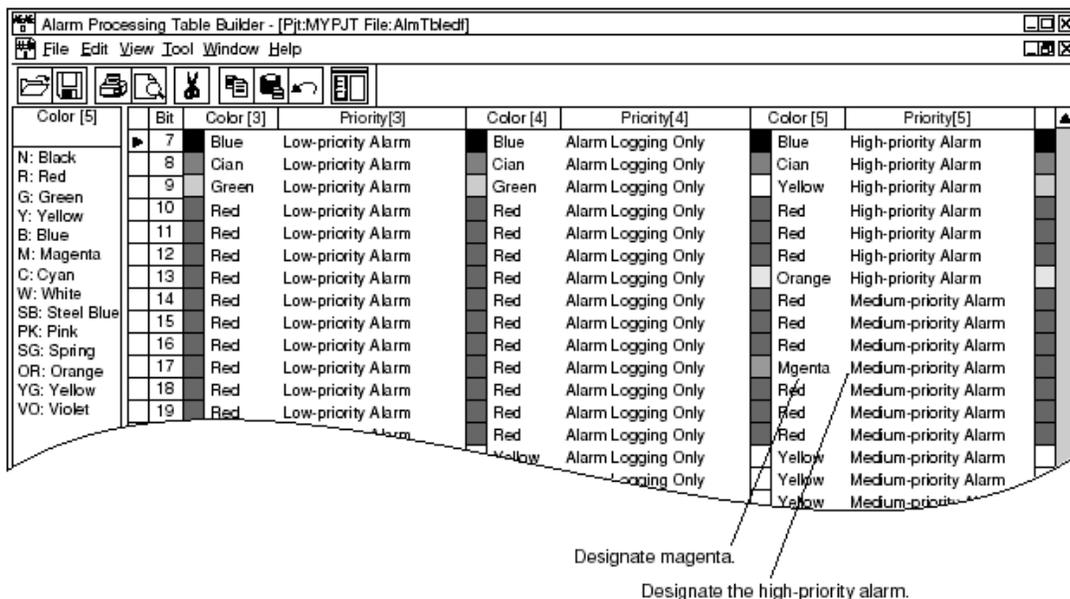
Figure: Designation in the Alarm Processing Table Builder
