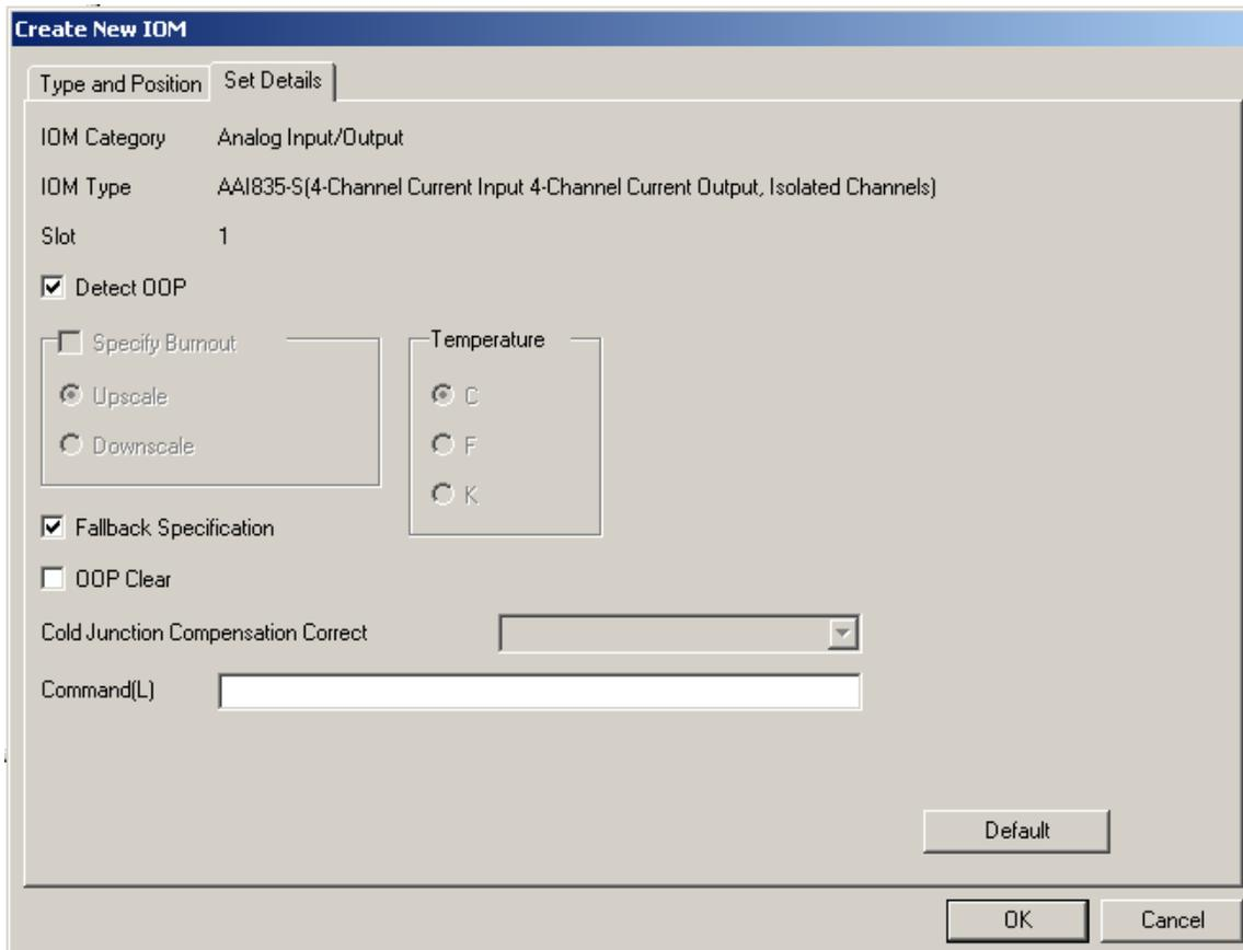
**Figure: Detail setting of a Analog input/output IOM**
