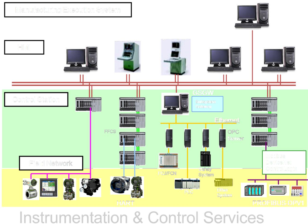
**Figure: CS3000 R3 System configuration**
