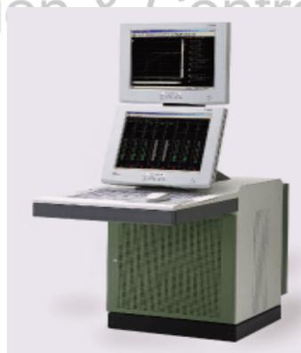
**Figure: Open display style console type of HIS**
