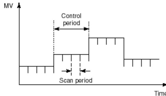
**Figure: The Control Period in the Regulatory Control Action**
