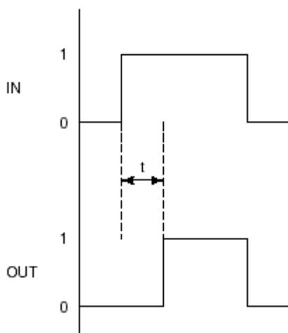
**Figure Behavior of On-Delay Timer**
