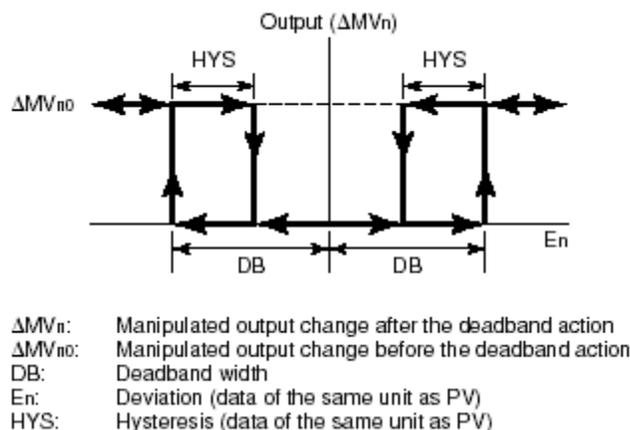
**Figure: Characteristics of Deadband Action**
