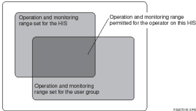
**Figure: Operation and Monitoring Range Permitted for Operator**
