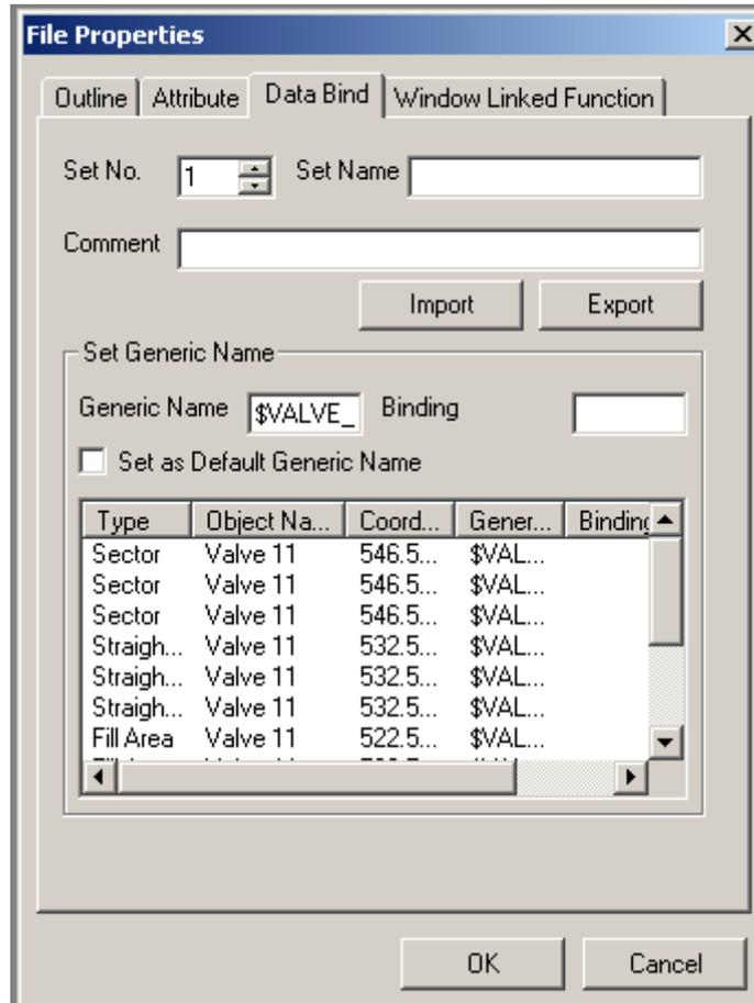
*Figure: Data bind tab of file properties*
