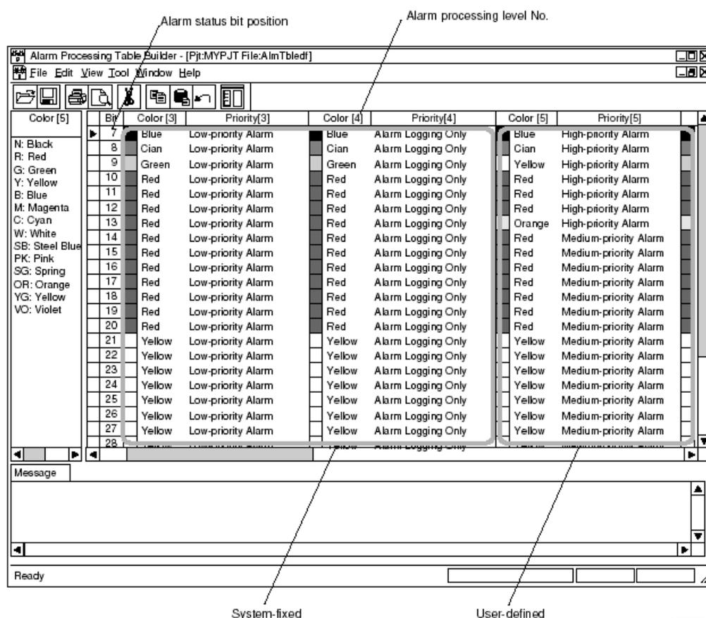
Figure: Alarm Processing Table Builder
