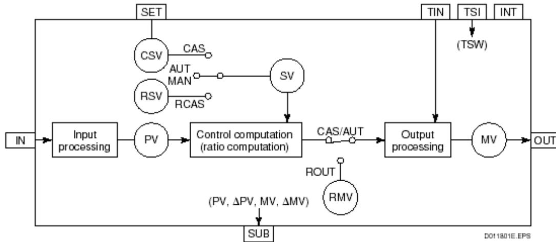
Figure: Function Block Diagram of Ratio Set Block (RATIO)
