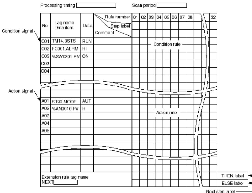
**Figure Conceptual Diagram of Complete Sequence Table**
