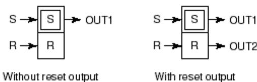
**Figure: SRS1-S and SRS2-S symbols**
