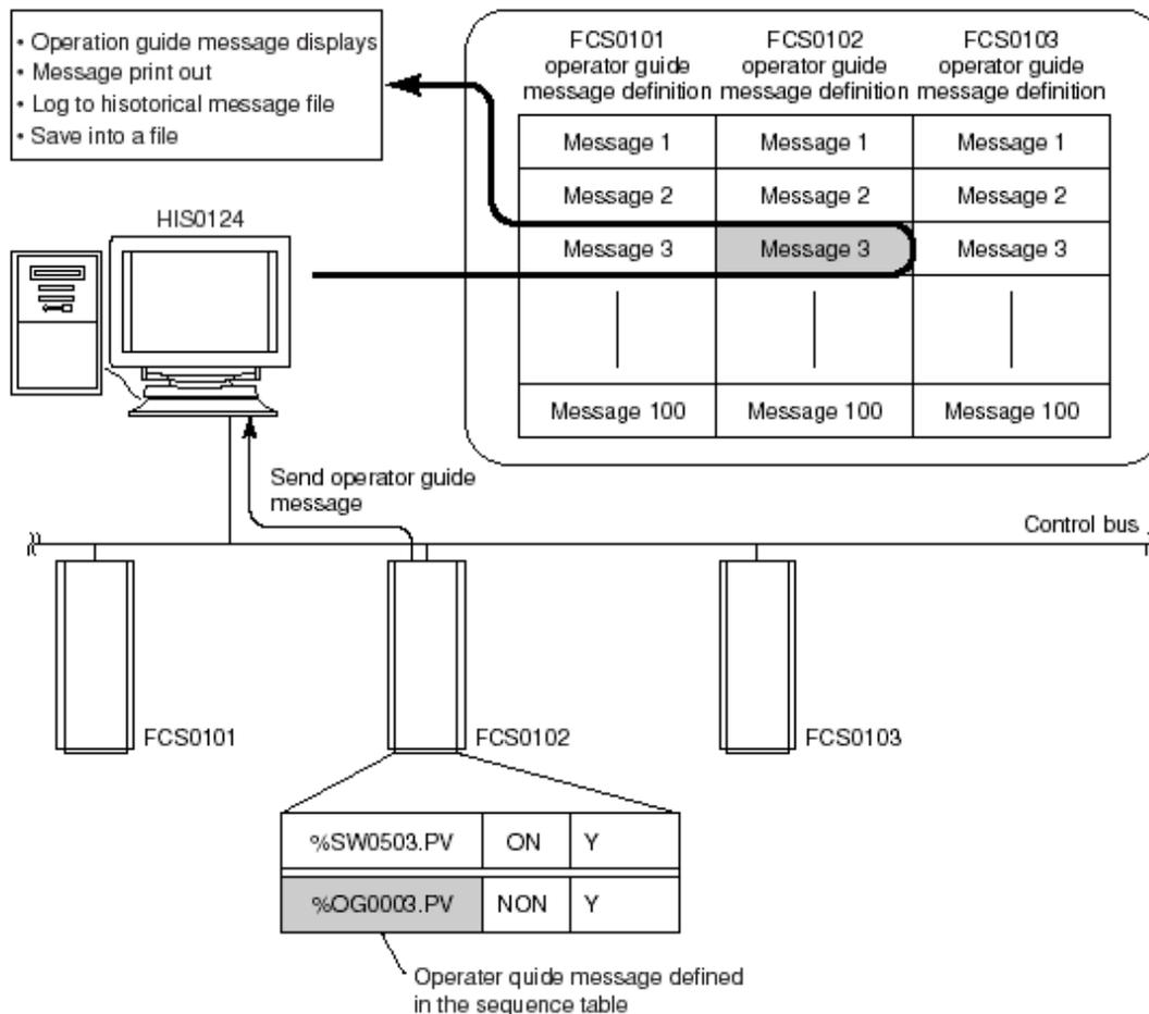
**Figure: Occurrence of an Operator Guide Message**
