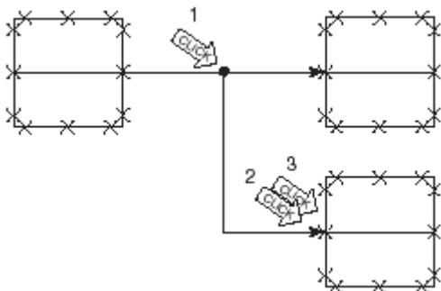
**Figure: Branching of wiring already drawn.**
