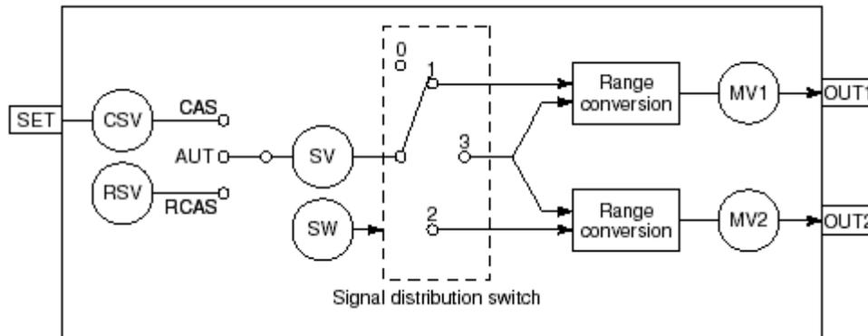
Figure: Function Block Diagram of Control Signal Splitter Block (SPLIT)
