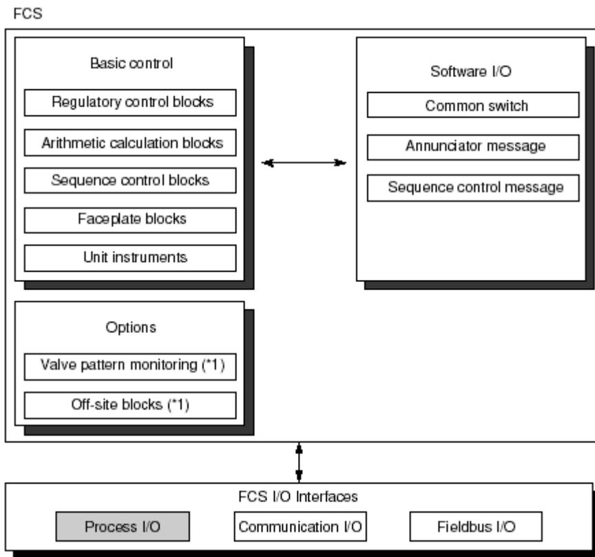
**Figure: Relationship of Process I/O with basic control**
