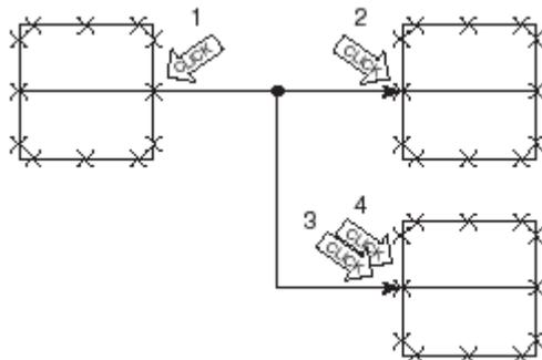
**Figure: Branching of wiring in Automatic wiring.**
