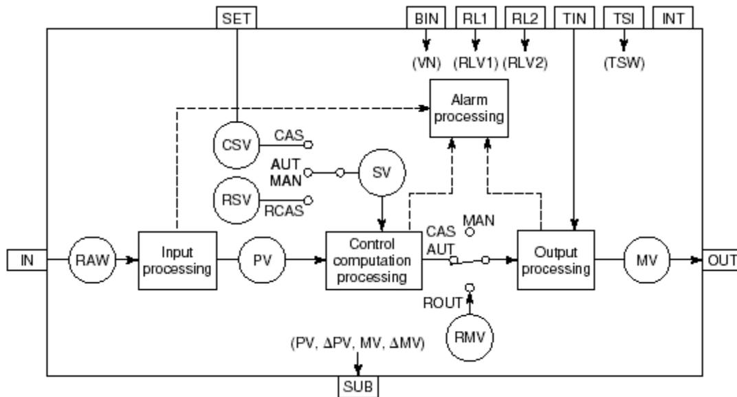
Figure: Function block diagram of a regulatory control function block.
