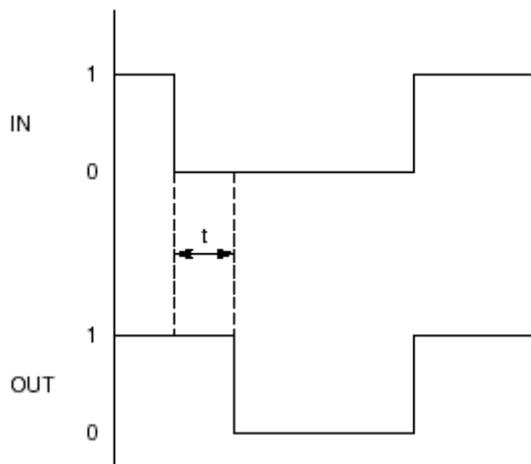
**Figure Behavior of Off-Delay Timer**
