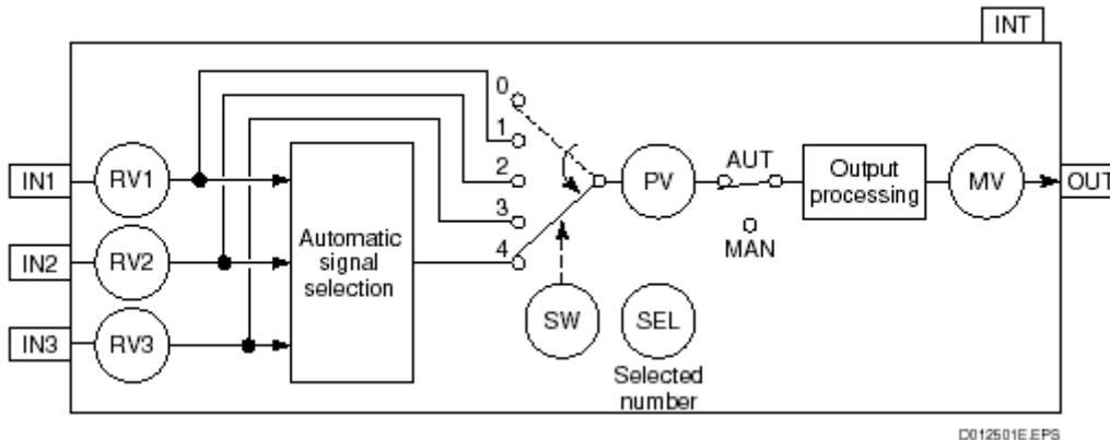
Figure: Function Block Diagram of Auto-Selector Blocks (AS-H/M/L)
