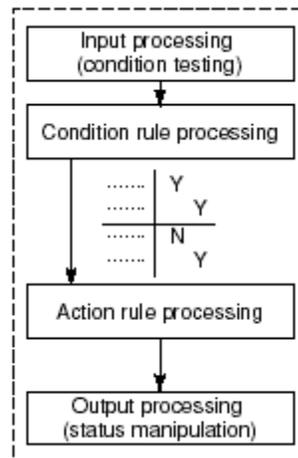
**Figure: Sequence Table Processing Flow**
