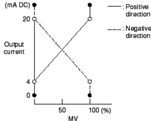
**Figure: Relationship between the Manipulated Output Value and Output Current**
