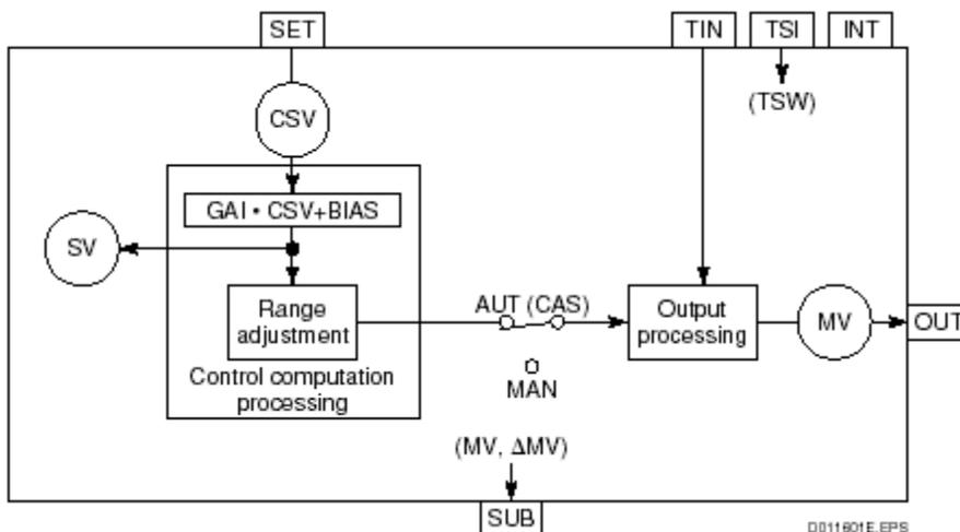
Figure: Function Block Diagram of Manual Loader Block with Auto/Man SW (MLD-SW)
