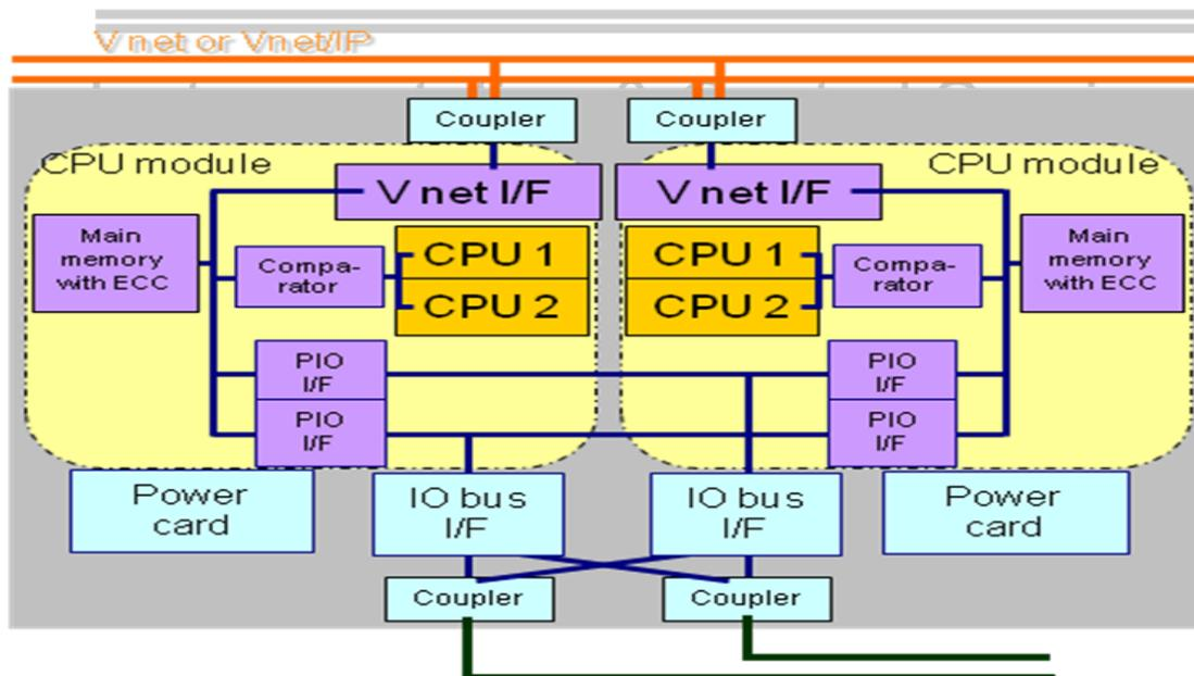
**Figure: Pair and Spare function of the CPU Card for FFCS.**
