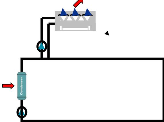
Water Cooled Heat Rejection System
