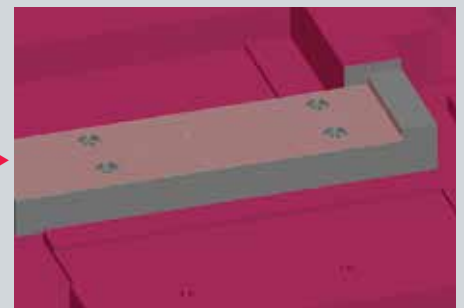
Selecting machining feature and deselecting protected surfaces
