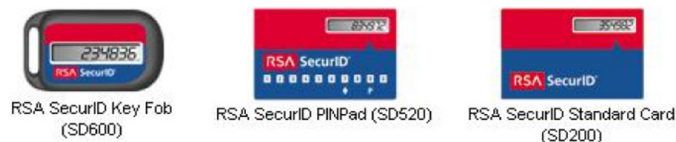
Figure 2.9: Illustrated are some of the hardware token-generating gizmos supplied by RSA Security for its SecurID "two-factor" authentication scheme, although the trend today is to use RSA-supplied software token schemes that can be installed on PCs, Palm Pilots, or even smart phones.
