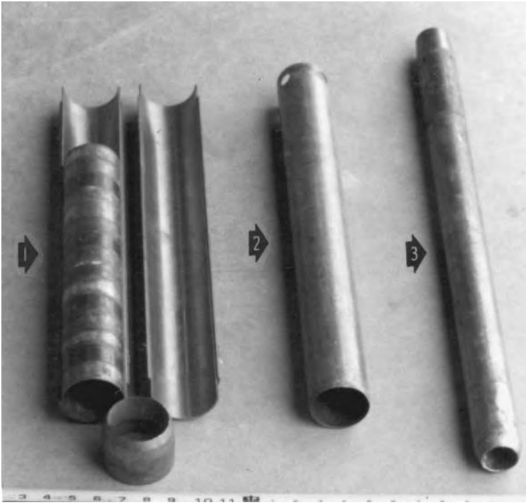
FIGURE 6.1 Soil Samplers (no. 1 is the California Sampler in an open condition, no. 2 is a Shelby Tube, and no. 3 is the Standard Penetration Test sampler.)
