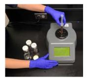
concentration in <u>parts per million</u>. Instead of using a light sensor to measure particles and report a unitless number, this instrument measures concentration and reports the results in parts per million. Using this method, there are no interferences with non-ferrous particles.
