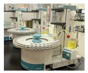
oil sample remains in the vial to eliminate interferences and contamination. Water content is determined via a reaction with iodine. The titration endpoint is reached when the instrument detects unreacted iodine. Results are reported as either percent water or parts-per-million (ppm). These units are easily converted by recognizing that 1% = 10,000 ppm. Other methods of detecting water may be more appropriate.
