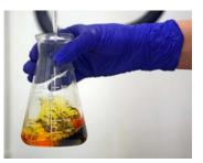
degrade oil properties and lead to corrosion of the internal components. The AN is lowest as a virgin oil and can gradually increase with use. High acid levels are typically caused by oil oxidation.
