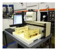
form of photons. A spectrum with different wavelengths is created for each element. The instrument quantifies the amount of energy emitted and determines the concentration in parts per million (ppm) of 20 elements present in the sample.
