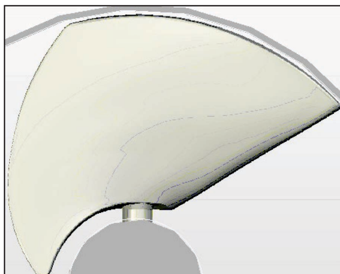
Figure 8 - Minimum clearance at optimal pitch
