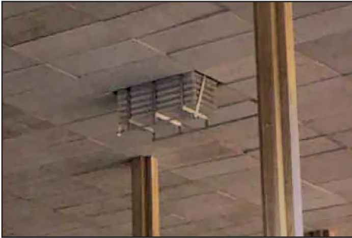
Figure 6 - Installation of a weighing basket in a cooling tower (Troncin, 2012)
