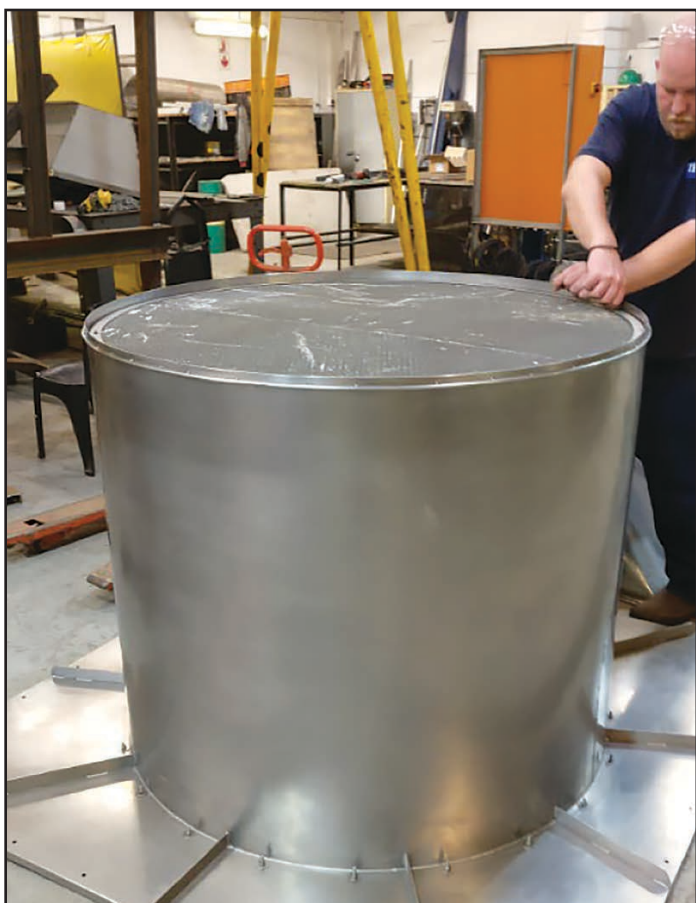
Figure 14 - Nozzle housing with honeycomb on the outlet
