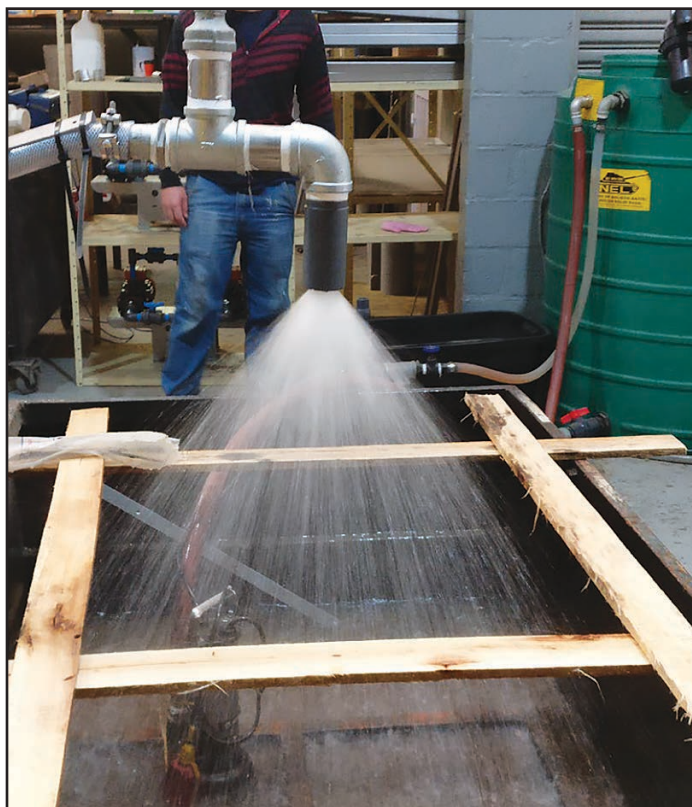
Figure 17 - Nozzle square spray pattern and distribution being measured and evaluated
