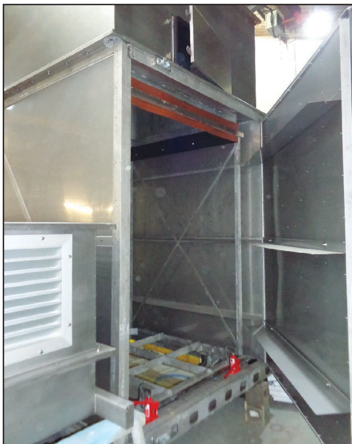
Figure 12 - Test section showing fill basket and bottle jacks
