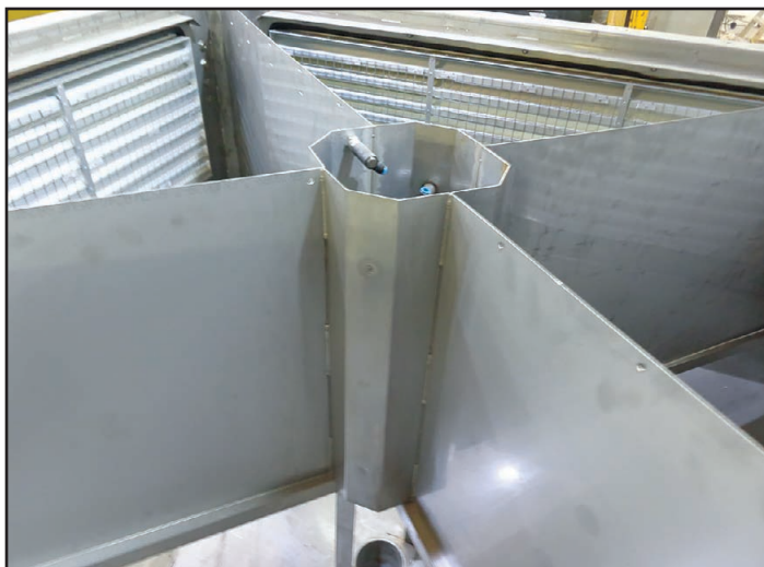
Figure 15 - Centre cross in the louver section with pressure taps
