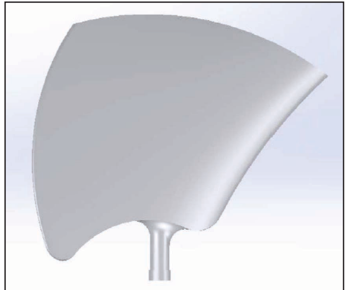
Figure 5 - Ultra low noise fan blade with leading edge and trailing edge swept according to a curved line
