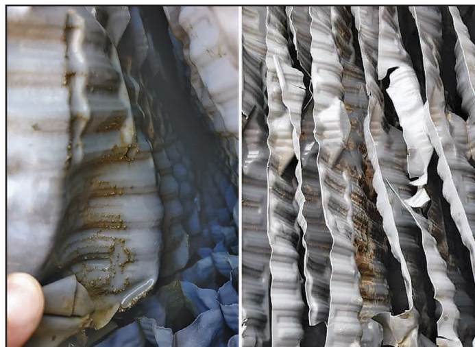
Figure 24 - Biological fouling starting to grow on the fill
