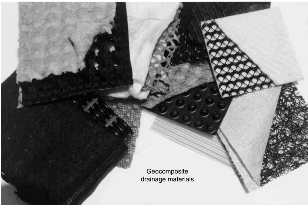
FIGURE 37.14 Typical geocomposite sheet drains.
