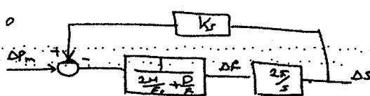
$$\Rightarrow \lambda_{1,2} = \frac{-D}{4H} \pm \sqrt{\frac{D^2}{4H^2} - \frac{2k_s \omega_0}{H}} = -\frac{D}{4H} \pm \frac{1}{2} \sqrt{\frac{D^2}{4H^2} - \frac{2k_s \omega_0}{H}}$$
