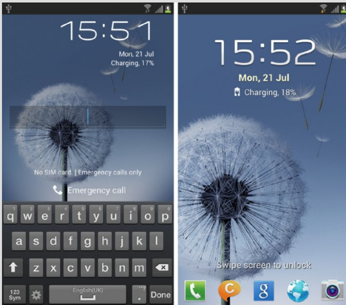
Figure 7.4 Device lock screen requiring a password and then this being removed after the exploit is run
