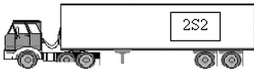
Figure 12: Picture of a FHWA class 7 (2S2) truck.
