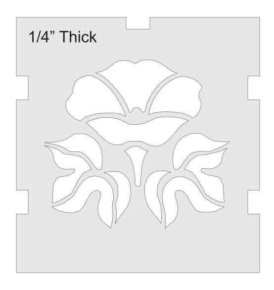
Take care to cut accurately when you cut the slot and tabs. You want the sides to fit together well. You can make up for some flaws by sanding.
