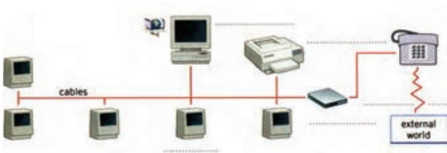
Figure 2: An example of a LAN
