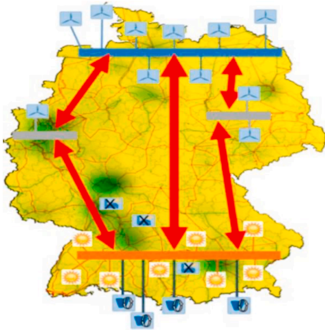
Fig. 9. The routes that need to be strengthened in the German transmission network [104].
