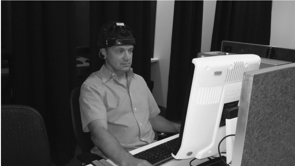
Figure 18.6b Experimental multimodal setup involving the use of dry electrode EEG device DSI-24 and Tobii T120 eye-tracking system (sampling rate: 120 Hz)
