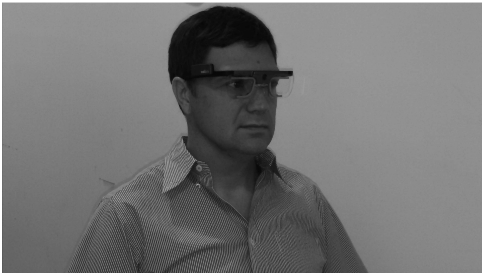
Figure 18.1a Portable eye-tracking device: Tobii Pro Glasses 2 (sampling rate: 50 Hz to 100 Hz)
