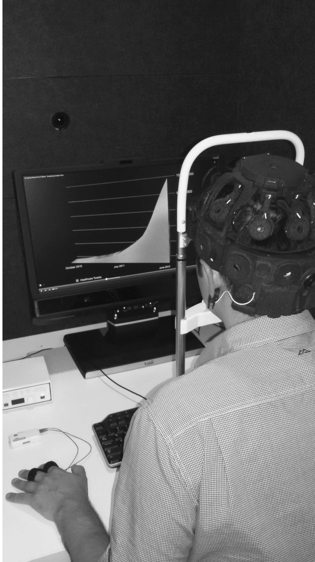
Figure 18.6a Experimental multimodal setup involving the use of dry electrode EEG device DSI-24, skin conductance device Shimmer3 GSR+, and Tobii TX300 eye-tracking system
