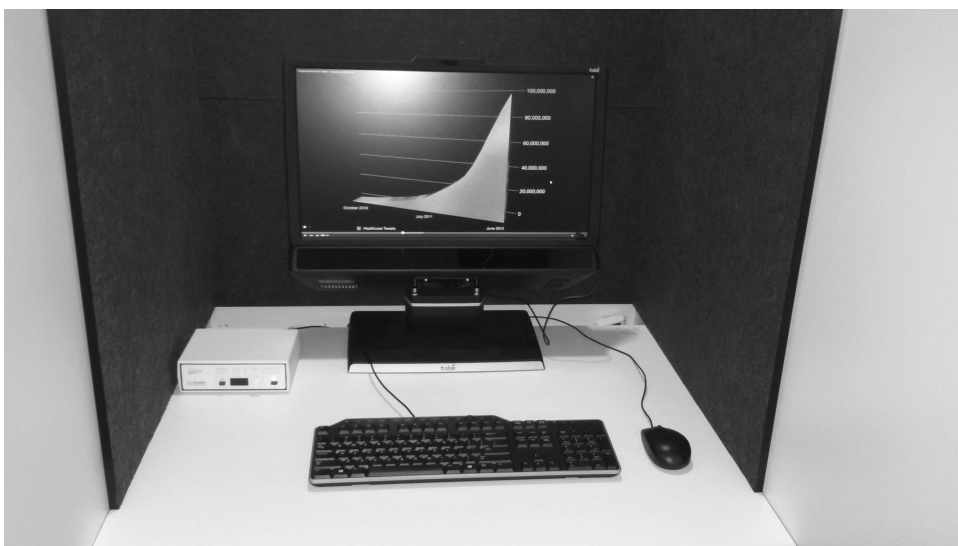
Figure 18.1b Stationary eye-tracking device: Tobii TX300 (sampling rate: 300 Hz)
