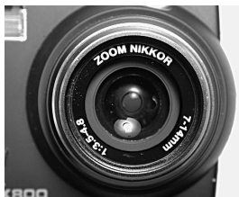
FIGURE 110. Focal length (7–14 mm) and f-ratio ( f/3.5 – f/4.8 ) (both variable on this zoom lens)
