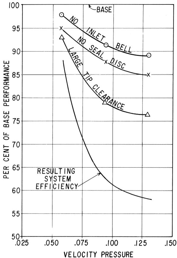
Figure 11. Results of Full Scale Fan Test.
