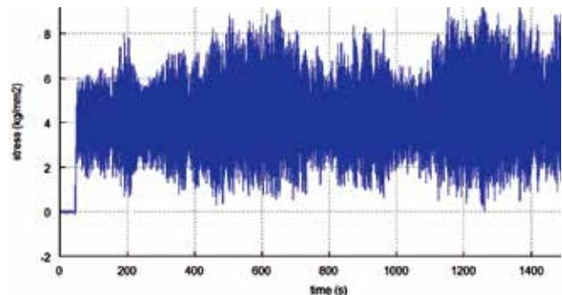
Fig. 8.2b: Stress recorded on Blade A (fixed speed)
