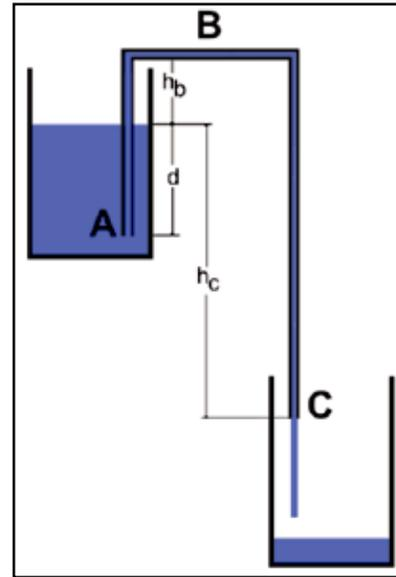
Figure 5: Siphon Principle
