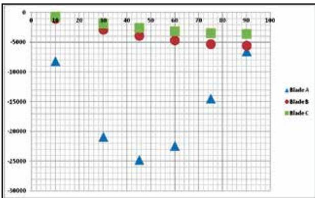
Fig. 5.1a: Blades max response (RBM fluctuation – N\*m)
