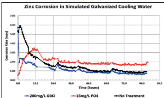
Figure No. 8 Corrosion rates for zinc in passivating water conditions.
