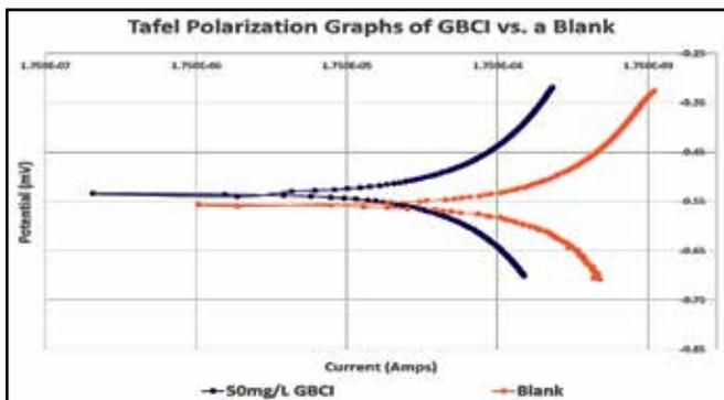
Figure No. 5 Tafel polarization plots of a GBCI treated electrode compared to an untreated electrode.
