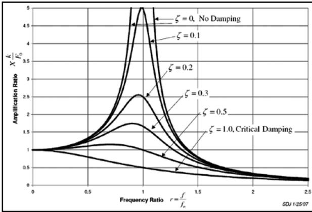
Fig. 7.1: SDOF response for various damping values (harmonic load)
