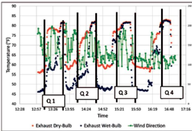
Figure 13: Exhaust measurements. 4 peaks show the 4 radii measured with some visual steps for the measurement starting from the outside of the fan stack. The first axis references the temperatures while the second axis is reference to the wind direction measured.
