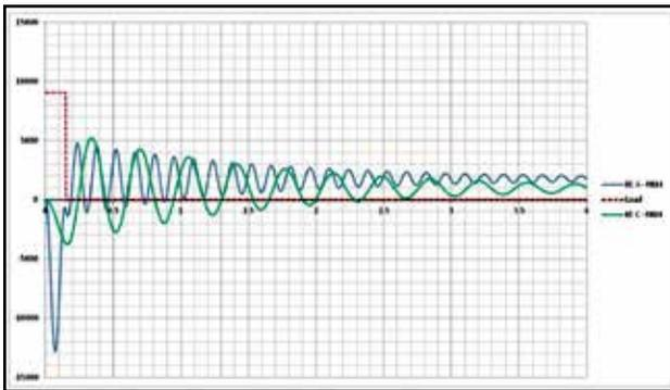
Fig. 4.3: Blades A & C response (RBM – N\*m) for AoC = 90°
