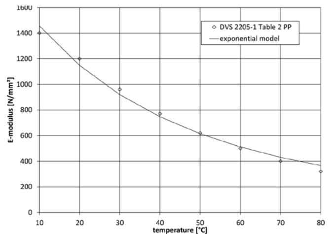
Figure 2: E-modulus of PP based on DVS 2205-1
