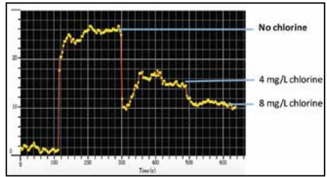
**Figure 3. Stability of TTA in the presence of high chlorine concentration**
