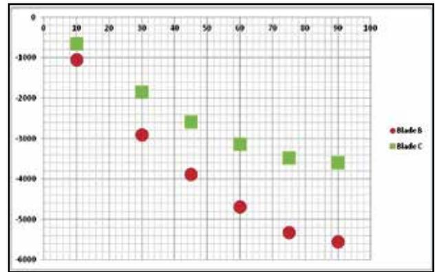
Fig. 5.1b: Detail of Fig. 5.1a - Comparison between Blade B and Blade C (RBM fluctuation – N\*m)
