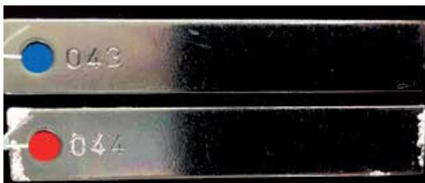
Figure No. 13 Front of galvanized coupons after one-week submersion in water Blue dot: 200mg/L GBCI | Red dot: no inhibitor
