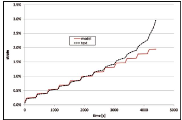
Figure 9: Comparison of the model with a test until failure
