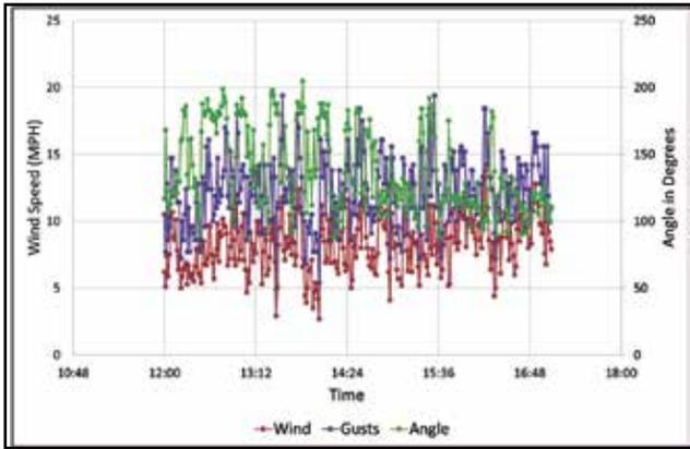
Figure 12: Time vs Wind Speed and Wind Direction. This 3-axis chart shows the wind speed average and gusts as well as the direction of wind measured by the wind station. The chart shows the highly inconsistent winds with respect to velocity and direction. A direction change can be denoted midway through of the test.
