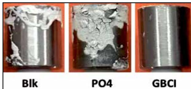
Figure No. 11 Zinc electrodes of various treatments in aggressive water conditions.
