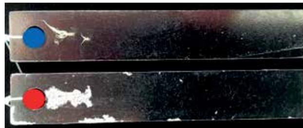
Figure No. 14 Back of galvanized coupons after one-week submersion in water. Blue dot: 200mg/L GBCI | Red dot: no inhibitor
