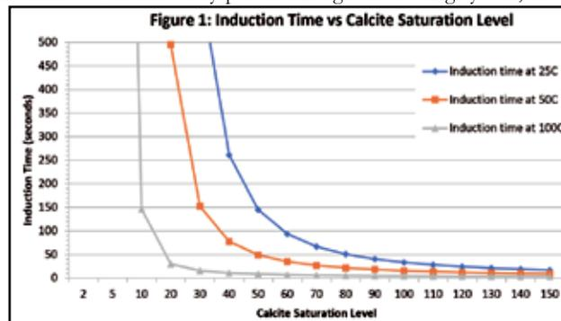
process adversely affected by scale. The induction time, in the absence of a scale inhibitor, has been modeled for common scales, including barite ( $BaSO_4$ ) and calcite ( $C_aCO_3$ ) for oil field brines. Figures 1 and 2 are derived from this study, and compared to related works.<sup>4</sup> The same laboratory procedures used to model induction time in oil field brines have been found to apply equally as well to cooling water and other scale forming systems.
