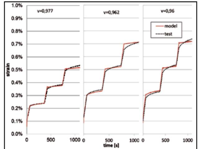
Figure 10: The fitted  $S_e$  (model and test data for different void ratios)
