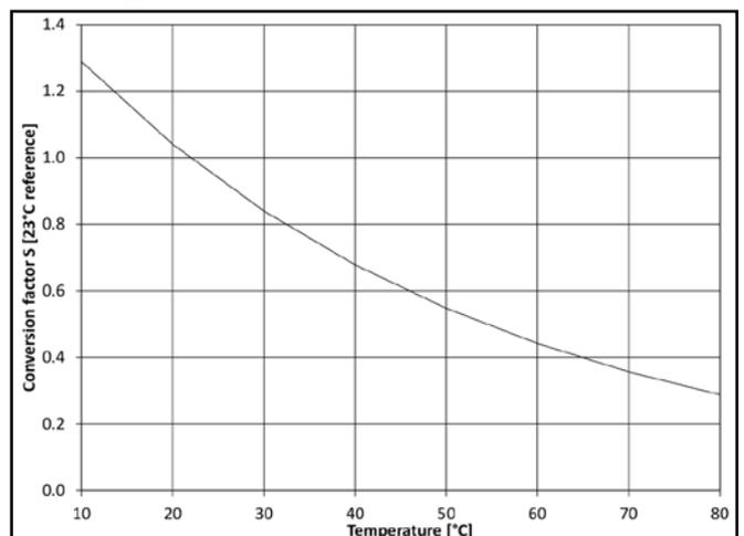
Figure 3: Temperature scaling factor S for PP based on DVS 2205-1
