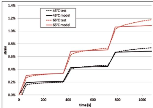
Figure 7: Step fit for elevated temperatures
