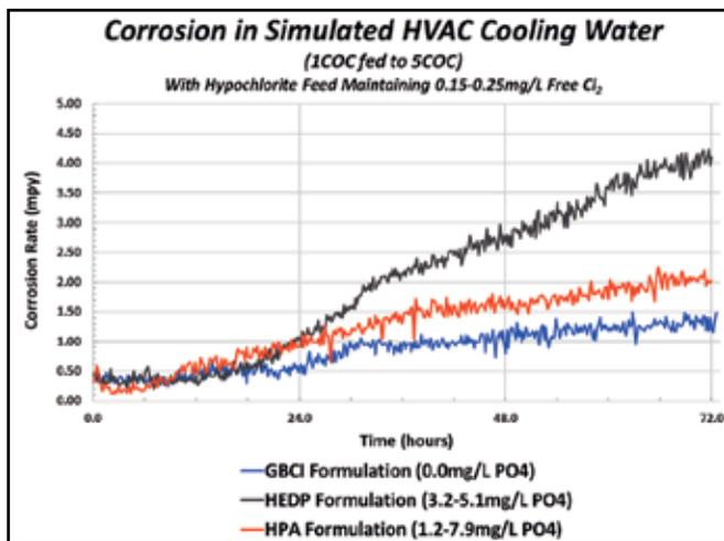
Figure No. 4 Corrosion test results of "low LSI" formulations in Simulated HVAC Water.
