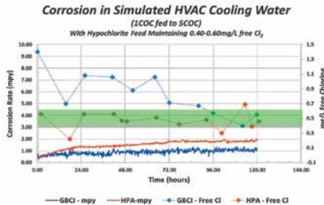
Figure No. 5 Corrosion test results of "low LSI" formulations in Simulated HVAC Water.
