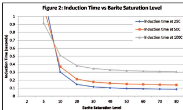
It should be noted that the induction times for both calcite and barite are several orders of magnitude below the typical residence time in an open recirculating cooling water system, oil field production process, or membrane
