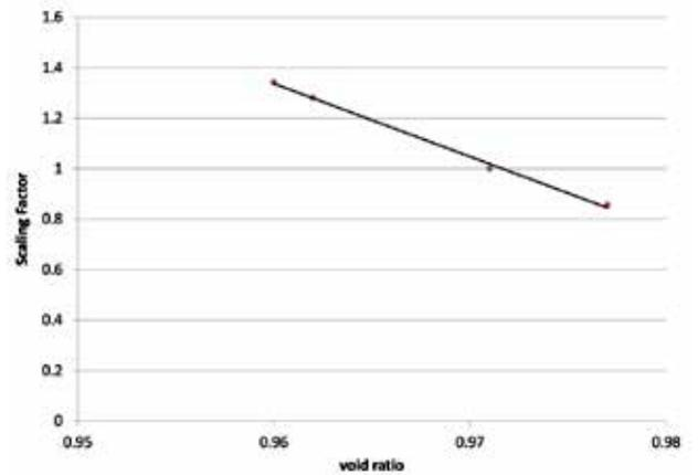
Figure 11: The fitted  $S_e$  for the corresponding void ratios (reference void ratio 0,971)
