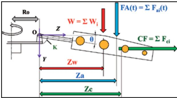
Fig. 3.1: Simplified Blade model and loads
