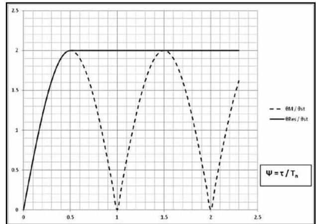
Fig. 4.1b: Maxima and Residual response spectrum of an un-damped SDOF system.
