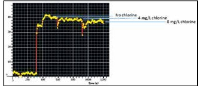
**Figure 4. Stability of HST in the presence of high chlorine concentration**
