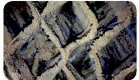
Scale embedded in biofilm on tower pack
