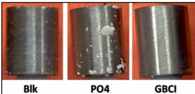
Figure No. 9 Zinc electrodes of various treatments in passivating water conditions.
