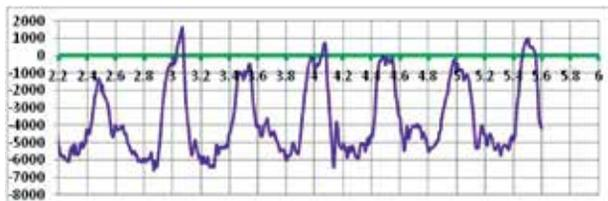
Fig. 2.4a: Load from high speed wind (Blade A)
