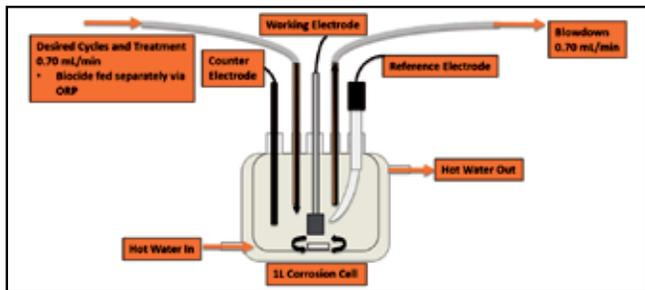
Figure No. 2 Modified corrosion cell with simulated cooling water feeds.
