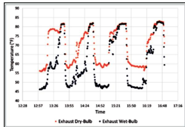
Figure 11: Time vs exhaust temperatures. The peaks represent the four distinct quadrant measurements. The trends show the difference in measurement between the early and later quadrants.
