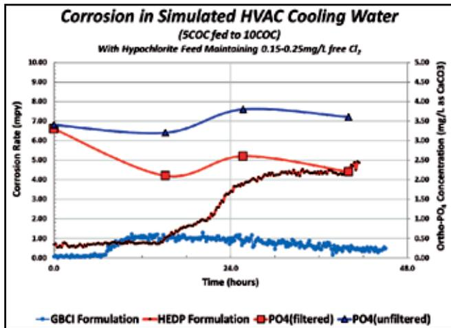
Figure No. 7 Corrosion test results of "high LSI" formulations in Simulated HVAC Water.
