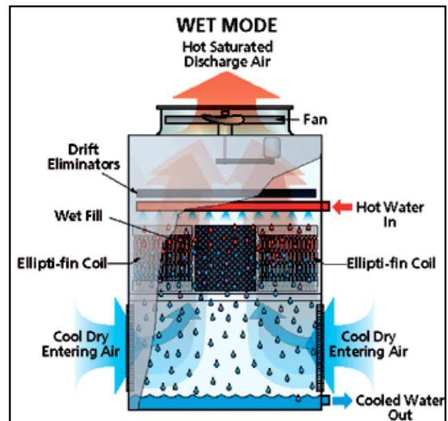
Figure 2: Wet Mode of Operation
