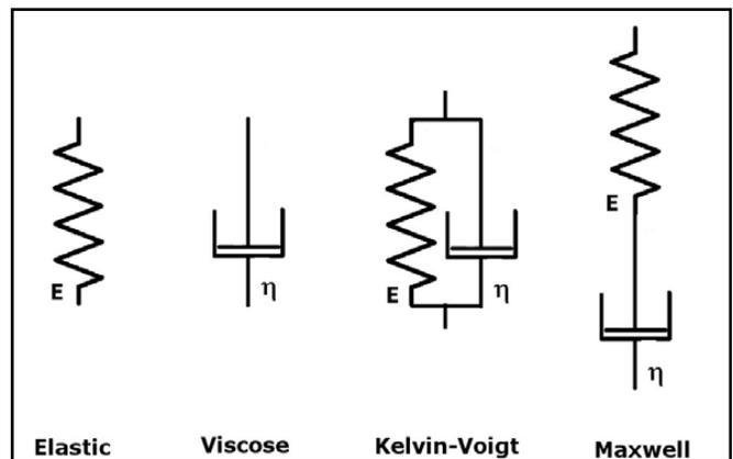
Figure 1: Linear viscoelastic model representations
