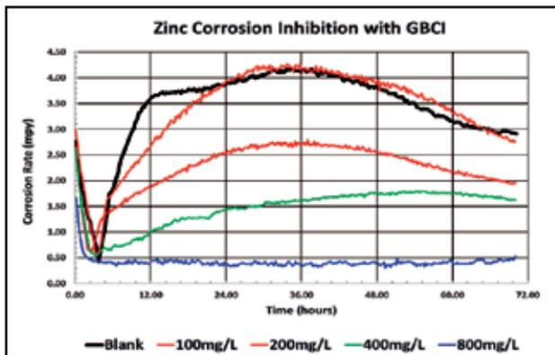
Figure No. 12 GBCI Dosage Curve for zinc metal in aggressive water conditions.
