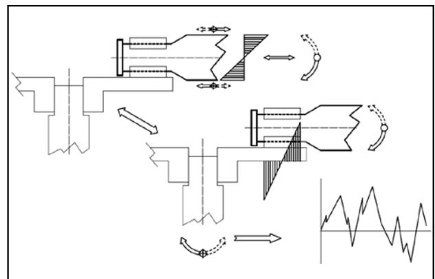
Fig. 6.1: RBM transmission to the drive chain and supporting structure
