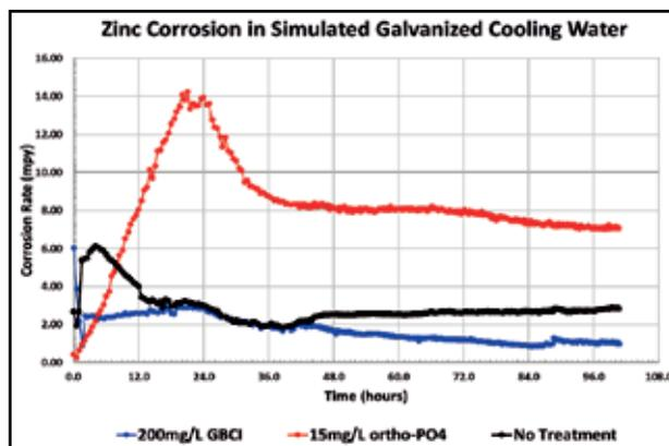
Figure No. 10 Corrosion rates for zinc in aggressive water conditions.
