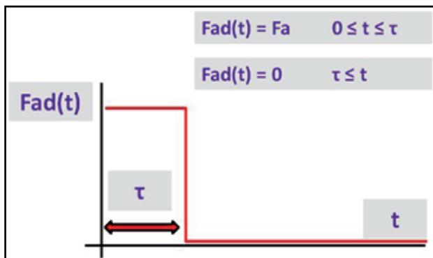
Fig. 4.1a: Rectangular step pulse
