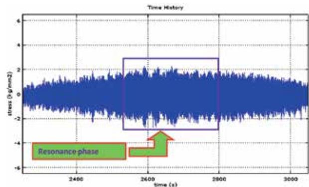
Fig. 8.2a: Stress recorded on Blade C (speed ramp)
