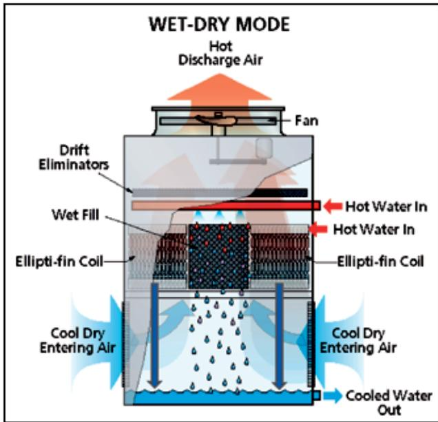
Figure 3: Wet-Dry Mode of Operation
