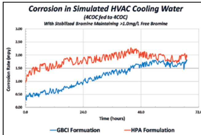
Figure No. 6 Corrosion test results of "low LSI" formulations in Simulated HVAC Water.
