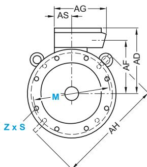
The motors are supplied with two fitted eyebolts conforming to IM B5, whereby one can be repositioned to conform to IM V1 or IM V3. It is important to note that stress must not be applied perpendicular to the ring plane.
