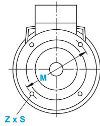
In DIN EN 50347, the frame sizes are allocated flange FF with through holes and flange FT with tapped holes. The designation of flange A and C according to DIN 42948 (invalid since 09/2003) are also listed for information purposes. See the table below. (Z = the number of retaining holes)
