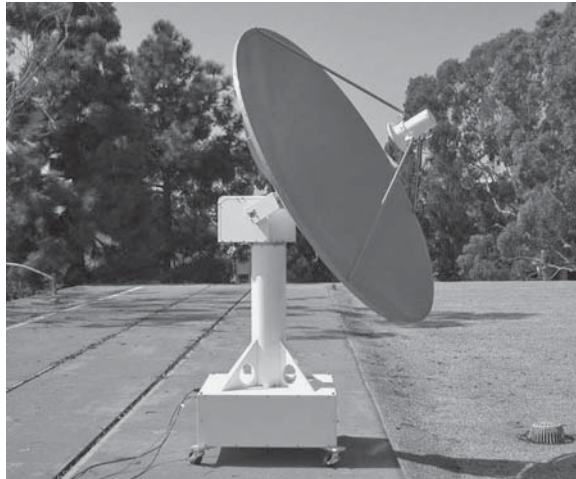
Figure 2-11 Antenna that uses program track techniques
