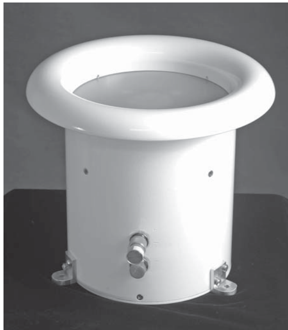
Figure 2-1 Rolled edge cavity antenna [4] (© 2004 IEEE)
