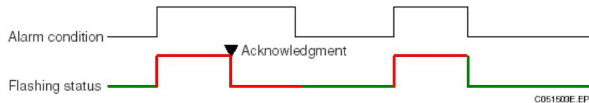
Figure Non-Locked Type Alarm Display Flashing Action
