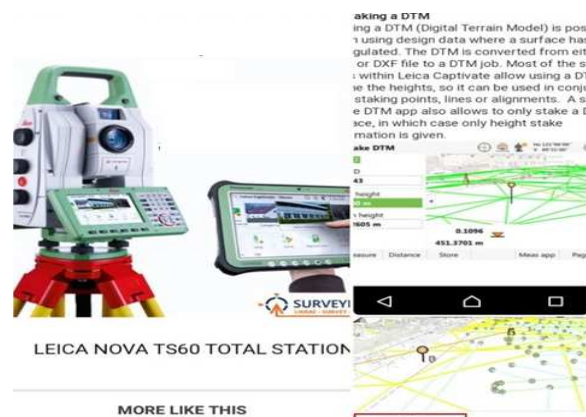
Fig.16 shows advanced TOTAL STATION whit DTM stakeout program
