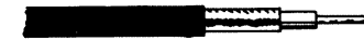
coaxial cable (From left to right: insulating jacket, woven outer conductor, low-loss insulating sleeve, inner conductor.)
