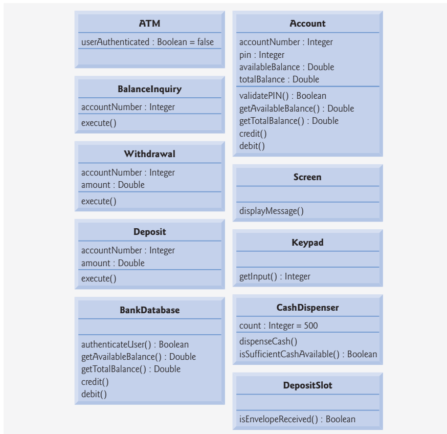
Fig. 6.21 | Classes in the ATM system with attributes and operations.
