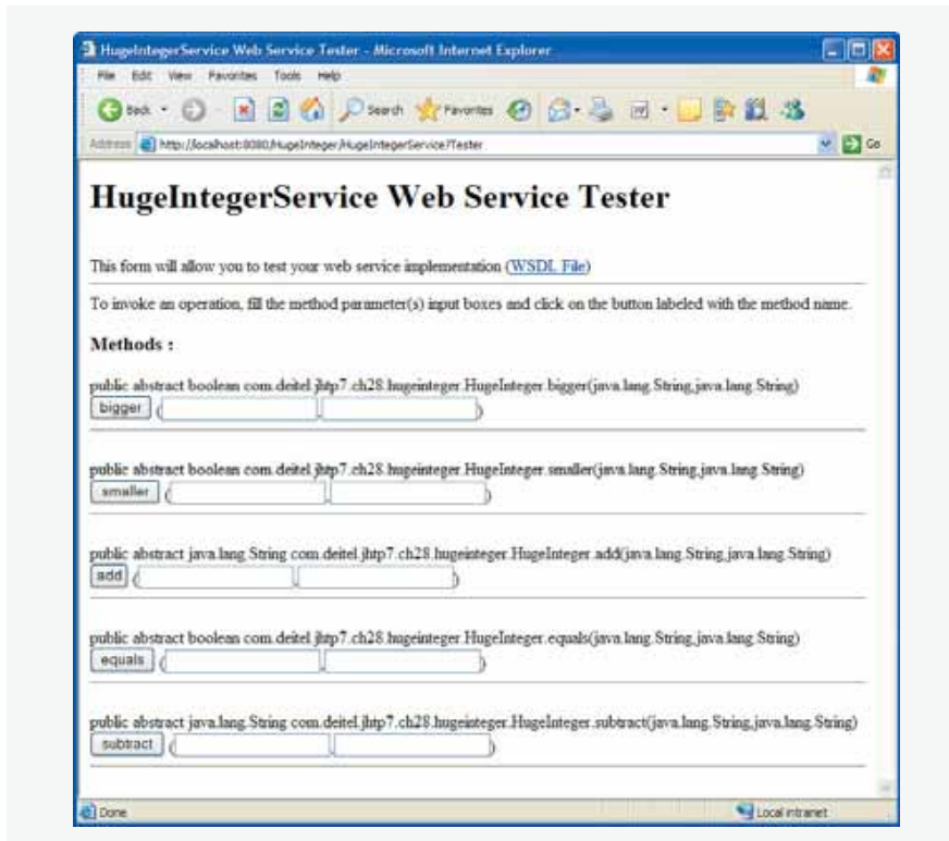
Fig. 28.4 | Tester web page created by Sun Java System Application Server for the HugeInteger web service.
