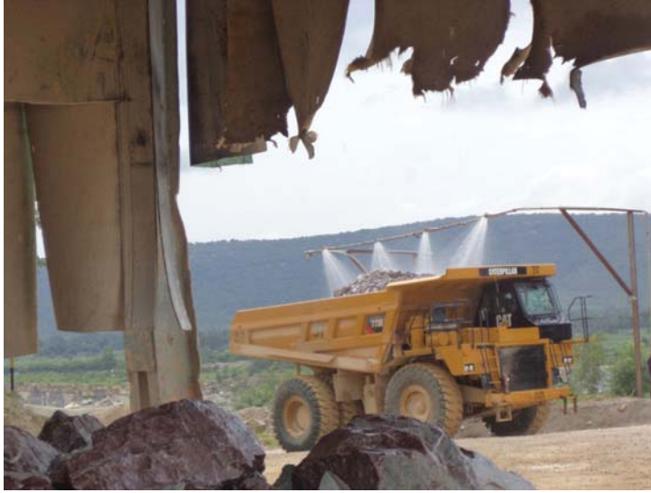
Figure 6.20 Water spraying to suppress dust during crushing.
