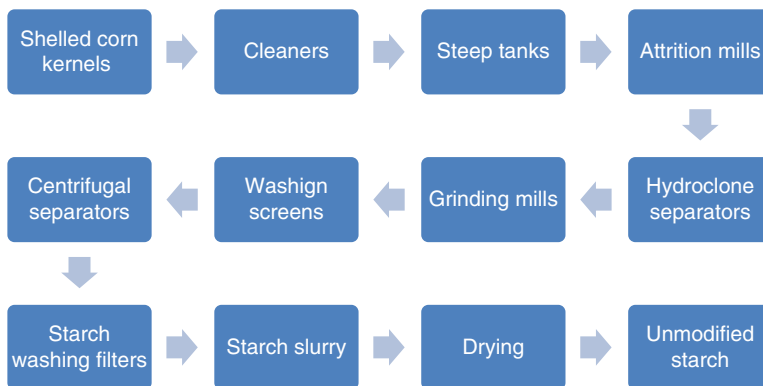
Figure 5.23 Schematic diagram of starch manufacturing from corn.
