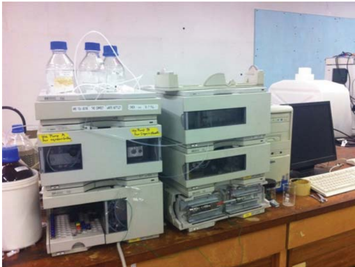
Figure 3.27 High-performance liquid chromatograph used to analyse nonvolatile chemical and biological compounds.
