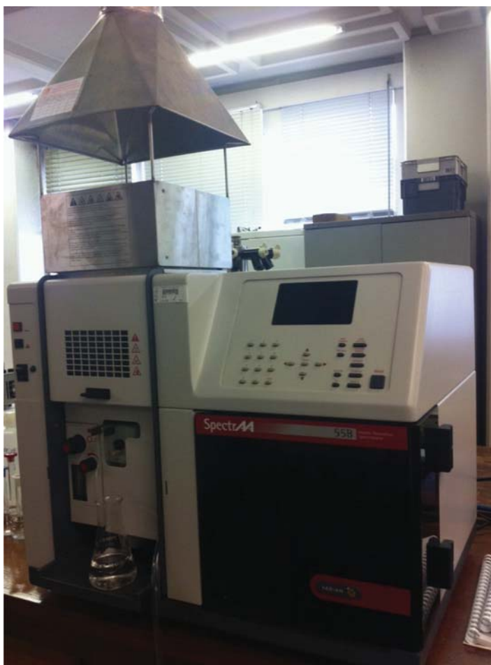
Figure 3.25 Atomic absorption spectrometer used to measure concentration of contaminants.
