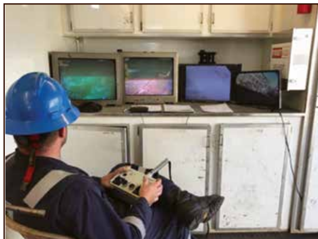
Figure 4 - Online robotic tank cleaning operator
