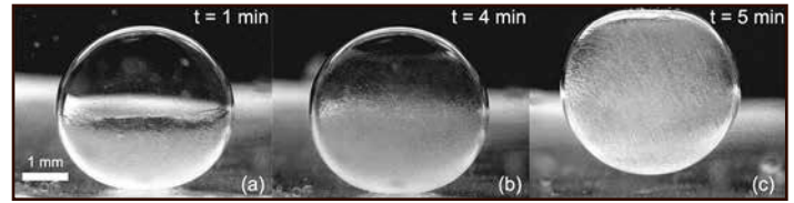
Figure 2. Frozen drop demonstrating low adhesion with a PTFE coated surface in a silicone oil bath. The drop passively detaches itself from the surface once the buoyancy force has exceeded the adhesive force. The ice layer grows upwards from the chilled substrate.
