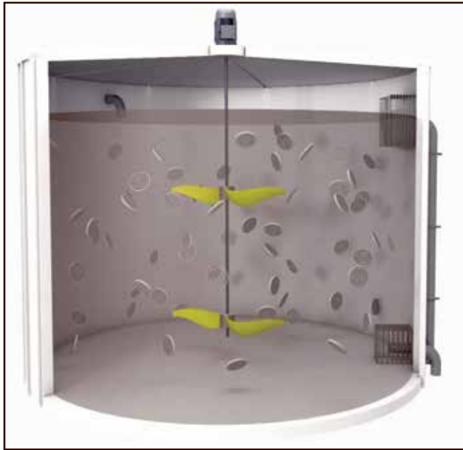
Figure 4. MBBR reaction vessel diagram showing mobile media.
