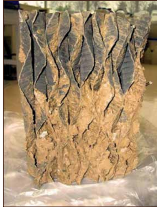
Figure 1. Fouled cooling tower film fill.
