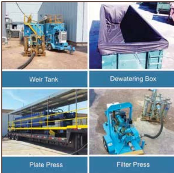
Figure 7 - Common dewatering methods used in online robotic tank cleaning
