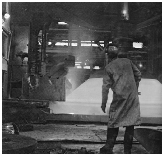
FIGURE 2.12 Forming a formed head in the mill.
