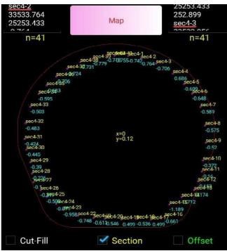
Fig.6 section was calculated and drawn Surveyor can control section of tunnel in app.
