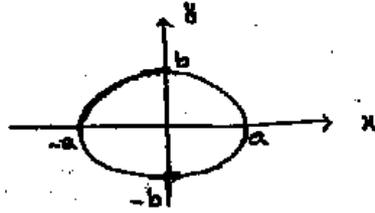
$$A = 2 \int_{-a}^a y \, dx = 2 \int_{\pi}^0 (b \sin t) (-a \cos t) dt = 2ab \int_{\pi}^0 \sin^2 t \, dt$$
