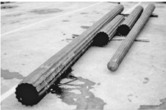
FIGURE 13.13 Raymond shell piles.
