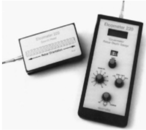
FIGURE 8.6 Shape of concrete cover thickness measurement machine.
