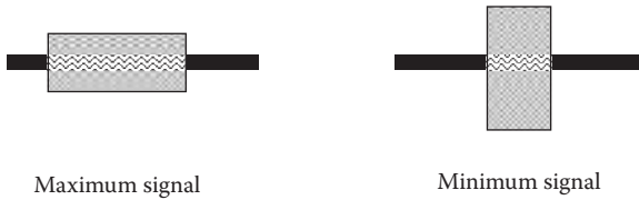
FIGURE 8.8 The correct device location.
