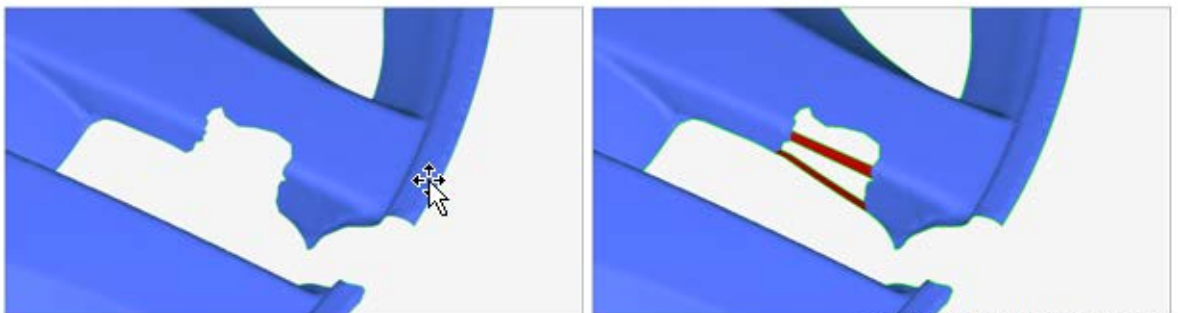
Figure 28: Damaged part/Bridge fill hole.
