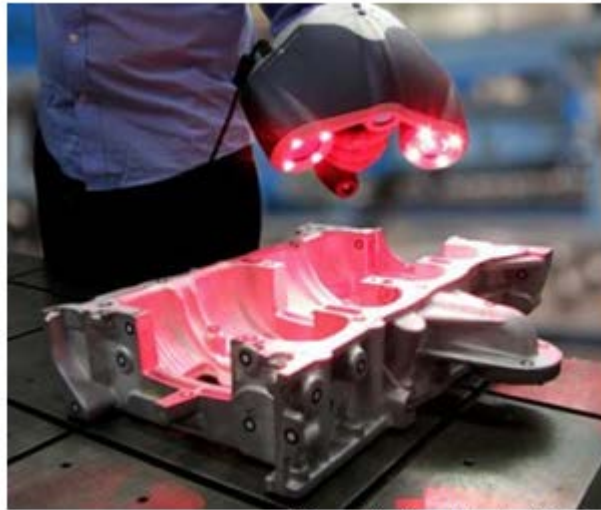
Figure 6: HandySCAN 3D scanner used to digitize a metal casting. The system uses stereo principle to simultaneously observe reflective markers (for positioning) and laser projection (for geometry detection).
