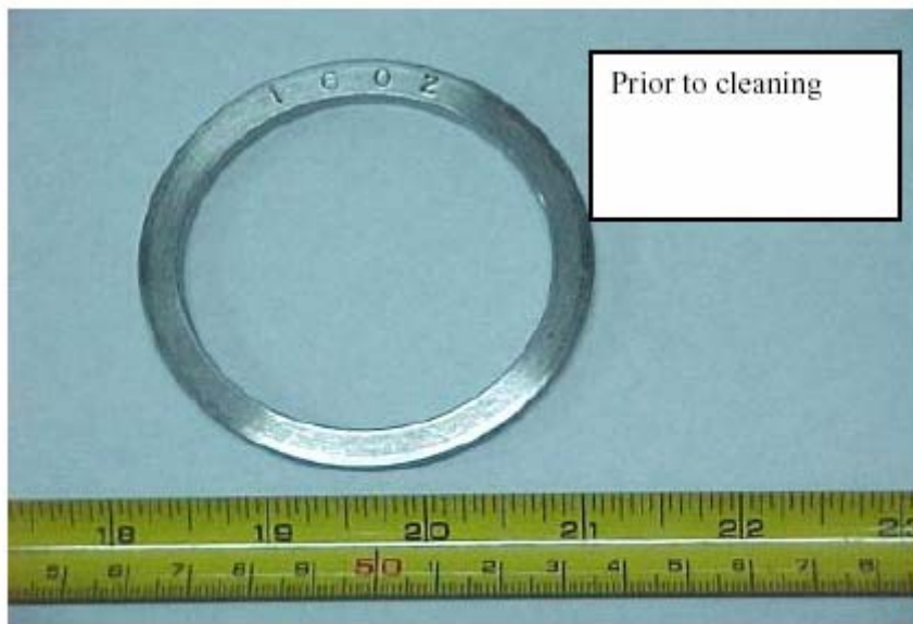
Figure 1. Condition of the corrosion coupon upon receipt in the lab
