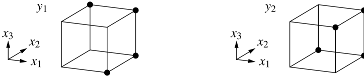
Fig. 5.6 Geometric interpretation of the function that is computed by a Fredkin gate (ignoring the input s which is simply passed through)
