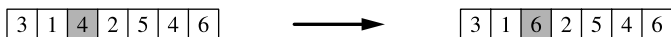
Fig. 12.10 Example of standard mutation: an allele of a gene is replaced by another allele
