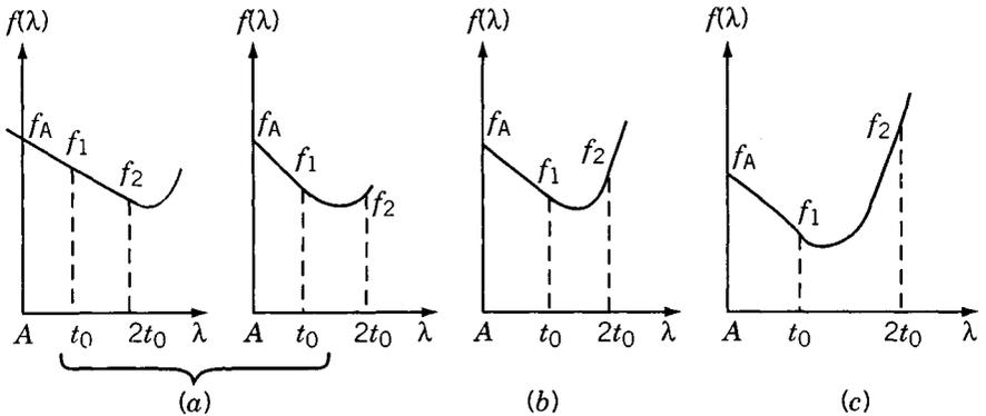
**Figure 5.14** Possible outcomes when function is evaluated at  $\lambda = t_0$  and  $2t_0$ : (a)  $f_2 < f_1$  and  $f_2 < f_A$ ; (b)  $f_2 < f_A$  and  $f_2 > f_1$ ; (c)  $f_2 > f_A$  and  $f_2 > f_1$ .
