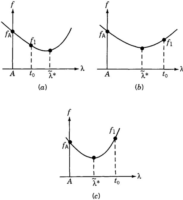
**Figure 5.13** Possible outcomes when the function is evaluated at  $\lambda = t_0$ : (a)  $f_1 < f_A$  and  $t_0 < \tilde{\lambda}^*$ ; (b)  $f_1 < f_A$  and  $t_0 > \tilde{\lambda}^*$ ; (c)  $f_1 > f_A$  and  $t_0 > \tilde{\lambda}^*$ .
