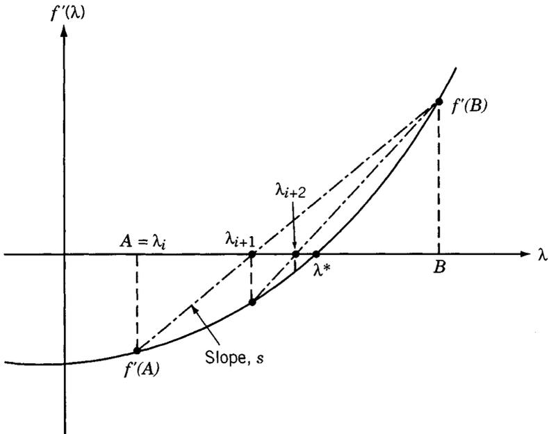
**Figure 5.19** Iterative process of the secant method.
